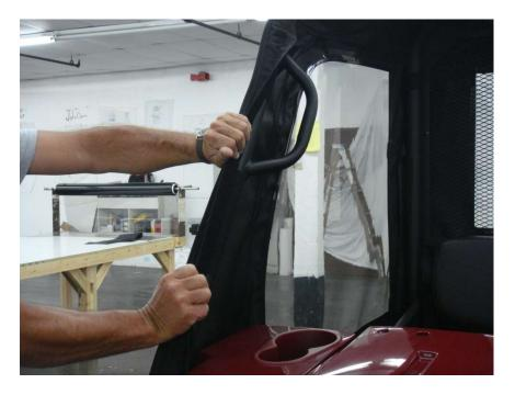
**Step 7:** The webbing/Velcro strip that runs the length of the front roll bars may need to be cut to accommodate the windshield clamps and the grab handle. With chalk, mark the webbing strip where cuts will be made. **DO NOT CUT INTO THE BINDING.**
