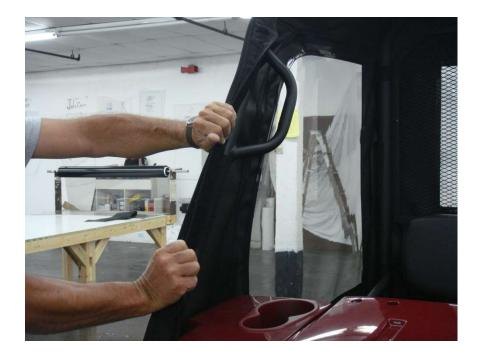
**Step 7:** The webbing/Velcro strip that runs the length of the front roll bars may need to be cut to accommodate the windshield clamps and the grab handle. With chalk, mark the webbing strip where cuts will be made. **DO NOT CUT INTO THE BINDING.**
