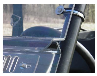
**Step 4:** When satisfied that the bottom windshield section is positioned properly, tighten the nuts on each clamp.
