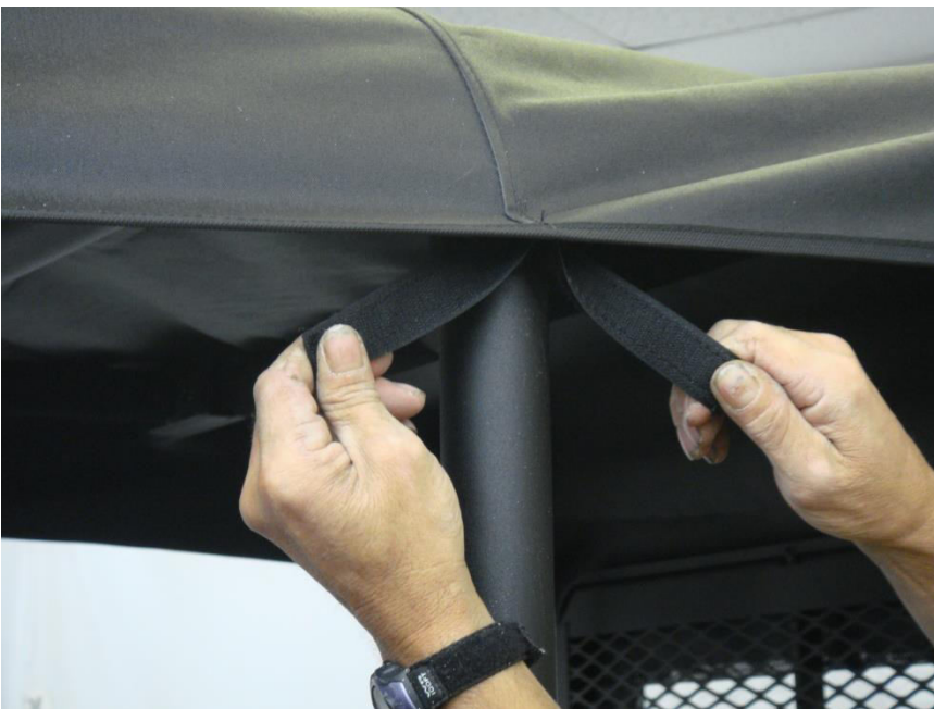
Figure 7.2 - attach 6" Center Roll Bar post enclosure Velcro Tabs to installed Velcro Strips
