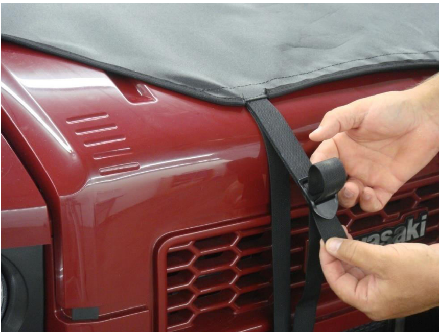
Figure 8.2 - Thread front Hood Strap into the buckles starting upward through the back of the buckle through the top opening
