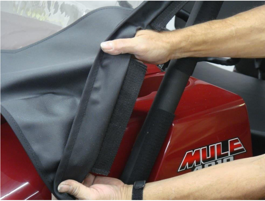
Figure 9.3 - attach bottom 8" Velcro Tabs to the installed Velcro Strips
