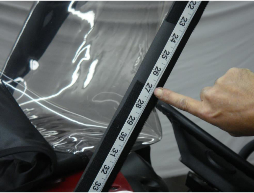
Figure 3.2 - install 8" Velcro Strip Vertically 27" below Roll Bar Cross-member weld joint
