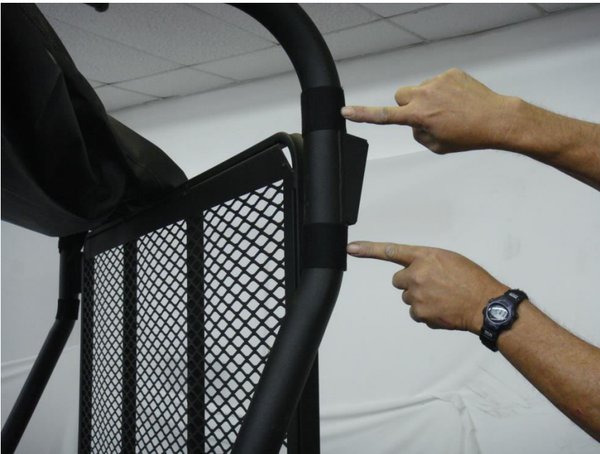
Figure 4.2 - Install 6" Velcro strips above and below the upright roll bar exhaust port
