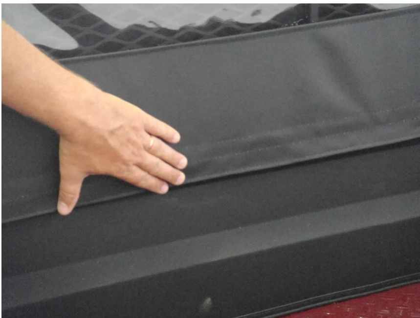
Figure 6.1 - square rear of enclosure to cab and attach rear enclosure Velcro tab to installed 46" Velcro strip
