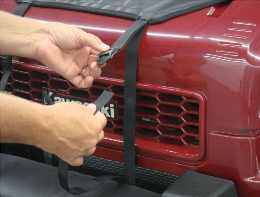
Figure 8.1 - Run Front Hood Straps around the Vehicle front bumper bar located behind the plastic Bumper Guard
