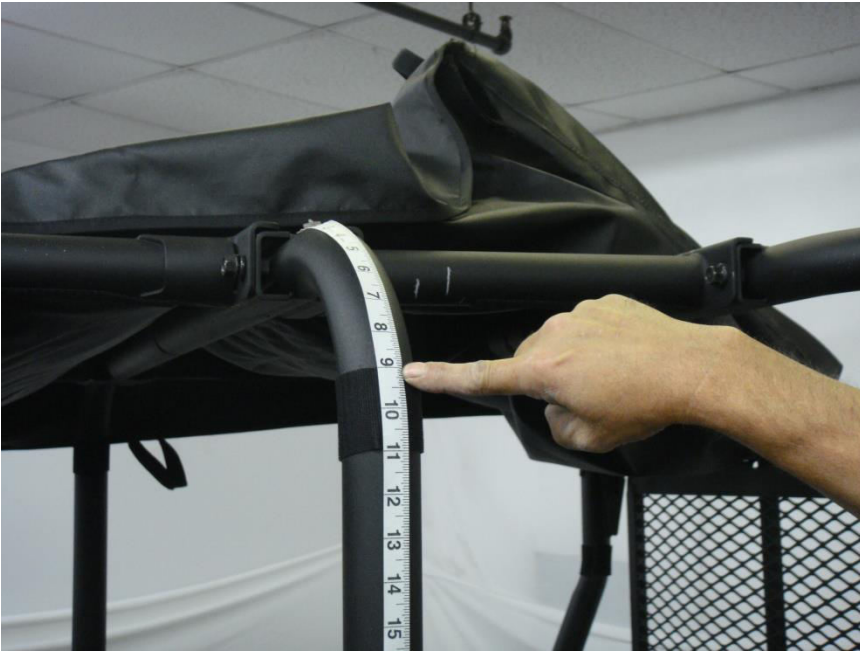
Figure 4.1 – install 6" Velcro strip horizontally around the Center Roll Bar upright 9" below the cross-member weld joint
