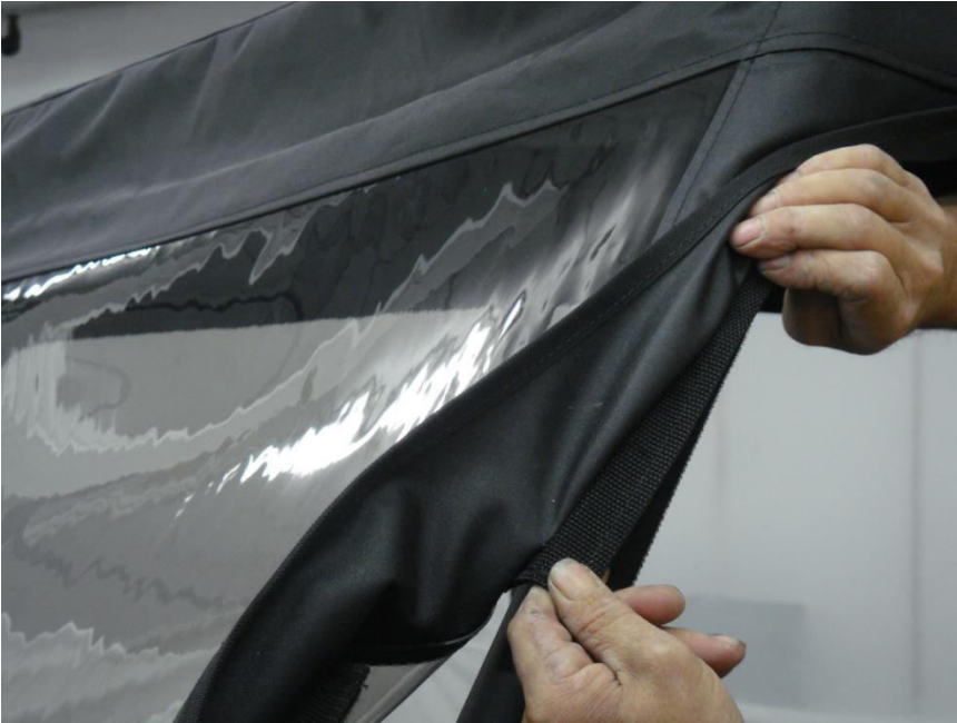
Figure 9.1 - attach top 8" Velcro Tabs to installed Velcro strips
