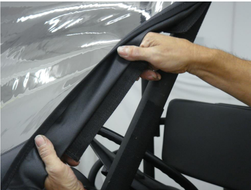
Figure 9.2 - Attach center 8" Velcro Tabs to installed Velcro strips
