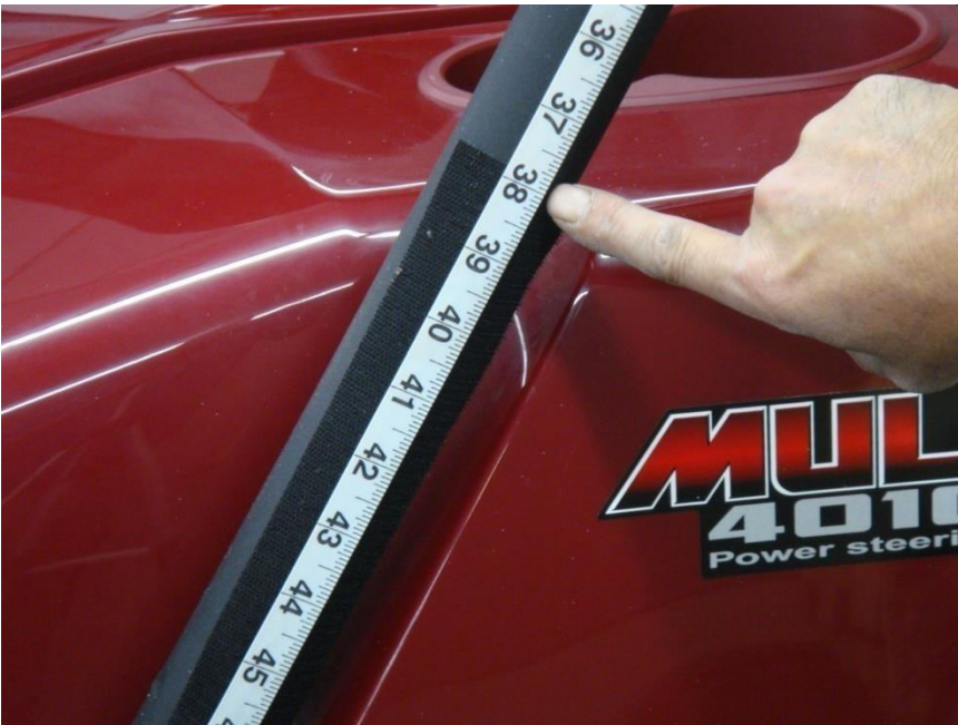
Figure 3.3 - install 8" Velcro strip Vertically 38" below Roll Bar Cross-member weld joint
