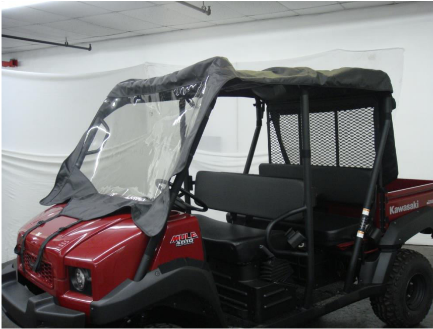
Figure 5.1 - place cab on top of vehicle cab roll bar and align seams to the center of corner roll bar tubes
