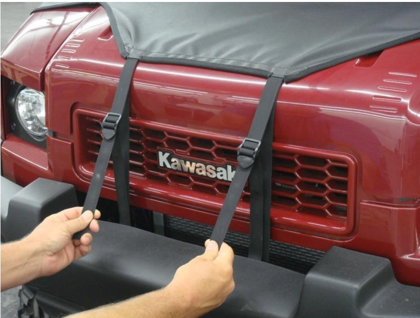
Figure 10.1 - tighten front hood straps until front windshields wrinkles are straightened out
