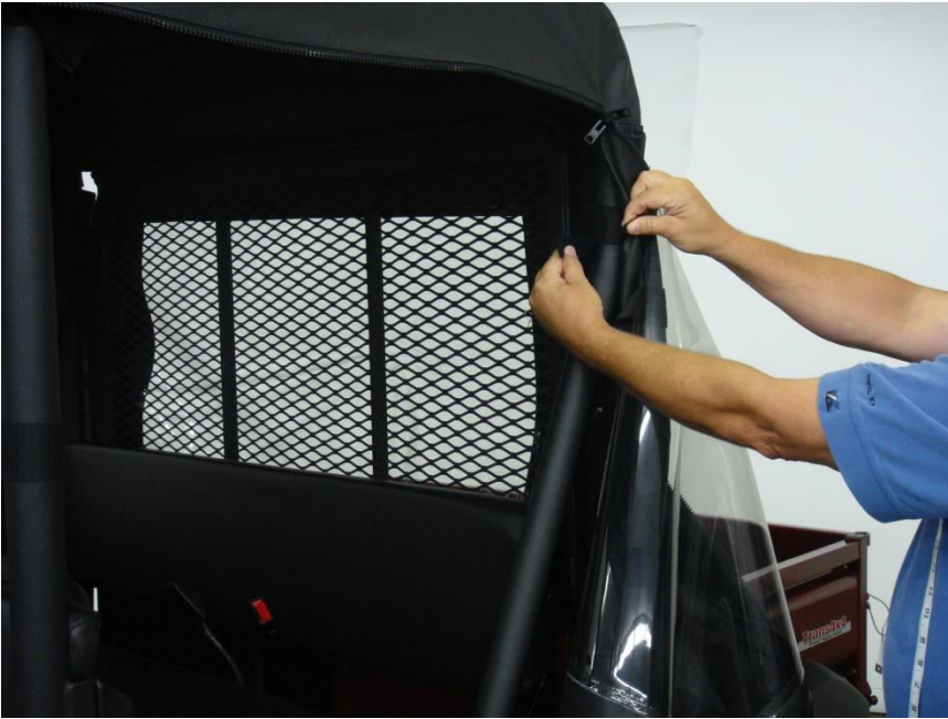
Figure 7.1 - attach 6" Rear Roll Bar post enclosure Velcro tabs to installed Velcro strips above and below the Roll bar exhaust port
