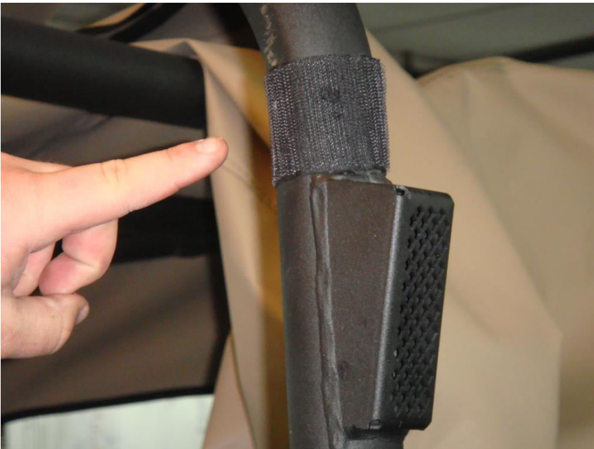
Figure 3.1 – place 6" Velcro strips horizontally around the rear Roll Bar post uprights just above the exhaust port
