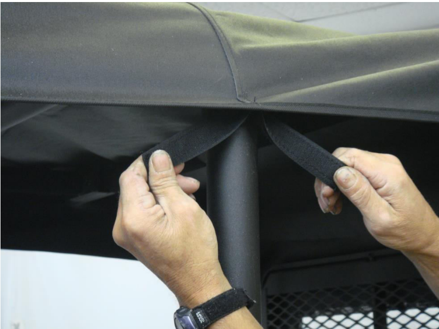
Figure 6.2 - attach Center Roll Bar Post upright Velcro tabs around installed Velcro strips
