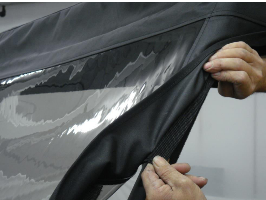
Figure 8.1 – attach top front Roll Bar Velcro Tab pulling outward and downward toward the front of the vehicle
