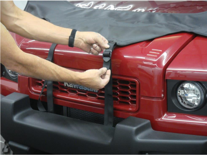
Figure 7.1 - run hood straps around the vehicle bumper and then latch through the buckle – secure but do not Fully Tighten at this time
