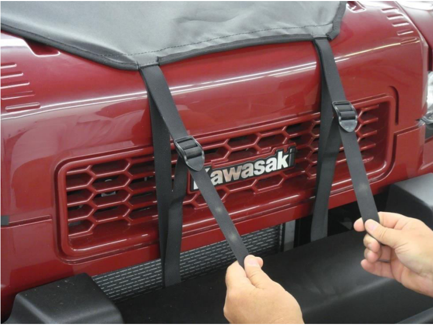
Figure 9.1 – fully tighten hood straps by pulling downward on both straps at the same time until front windshield is tight
