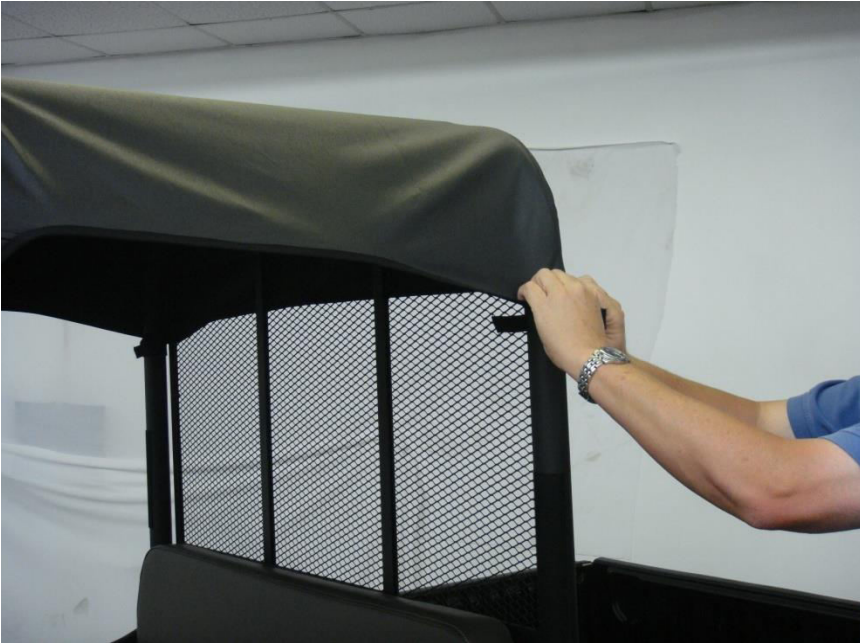
Figure 6.1 - attach Rear Roll Bar Post Velcro Tabs around installed Velcro strips
