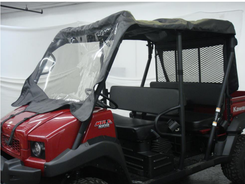
Figure 5.1 - Place enclosure loose on vehicle Cab Roll Bar Structure – Hood Straps to the front of the vehicle
