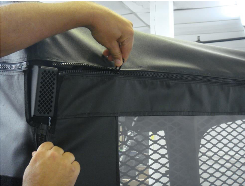
Figure 7.2B – attach Rear Window Panel by zipping it to the Top and Door Panels. Note Rear Roll Bar Exhaust port must be exposed
