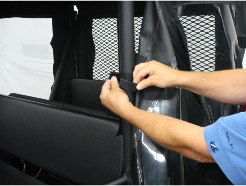
Figure 10.1 - attach Center Roll Bar upright enclosure tabs to installed 6" Velcro strips at the center and top of the Roll Bar Upright
