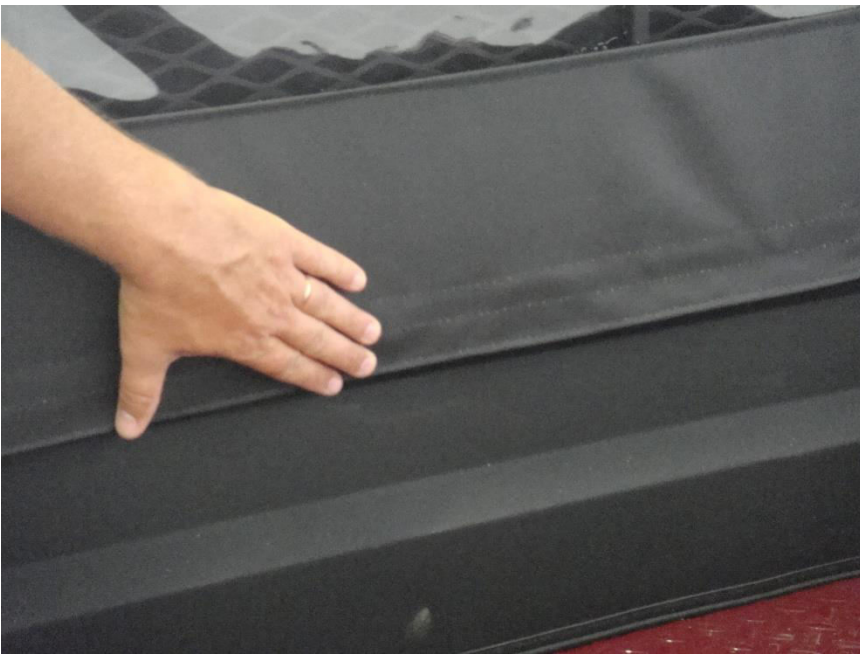
Figure 8.1 - square rear of enclosure to cab and attach rear enclosure Velcro tab to installed 46" Velcro strip
