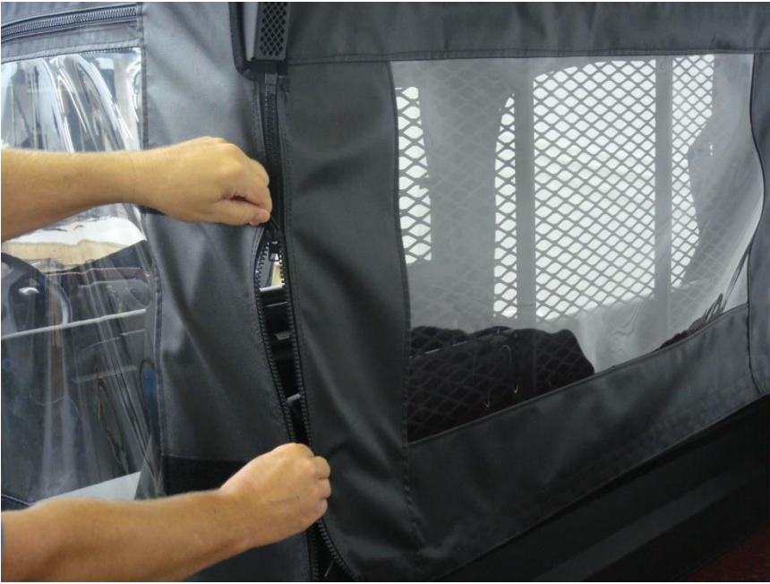
Figure 7.2A - attach Rear Window Panel by zipping it to the Top and Door Panels. Note Rear Roll Bar Exhaust port must be exposed
