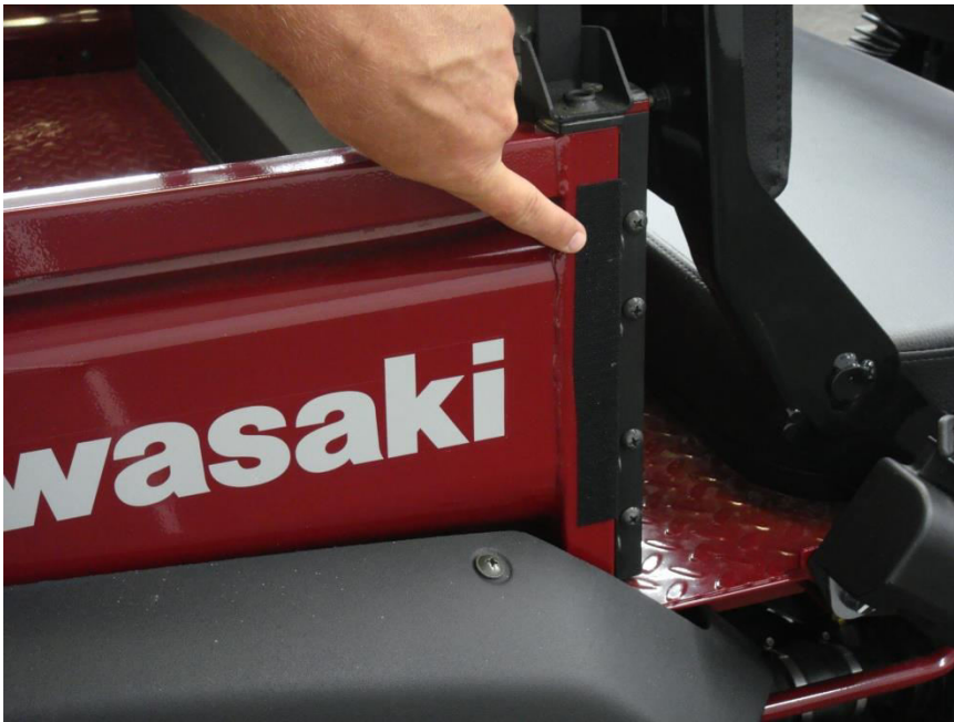
Figure 6.1 – install 10” (1” wide) Velcro Strips vertically to the Cargo Bed
