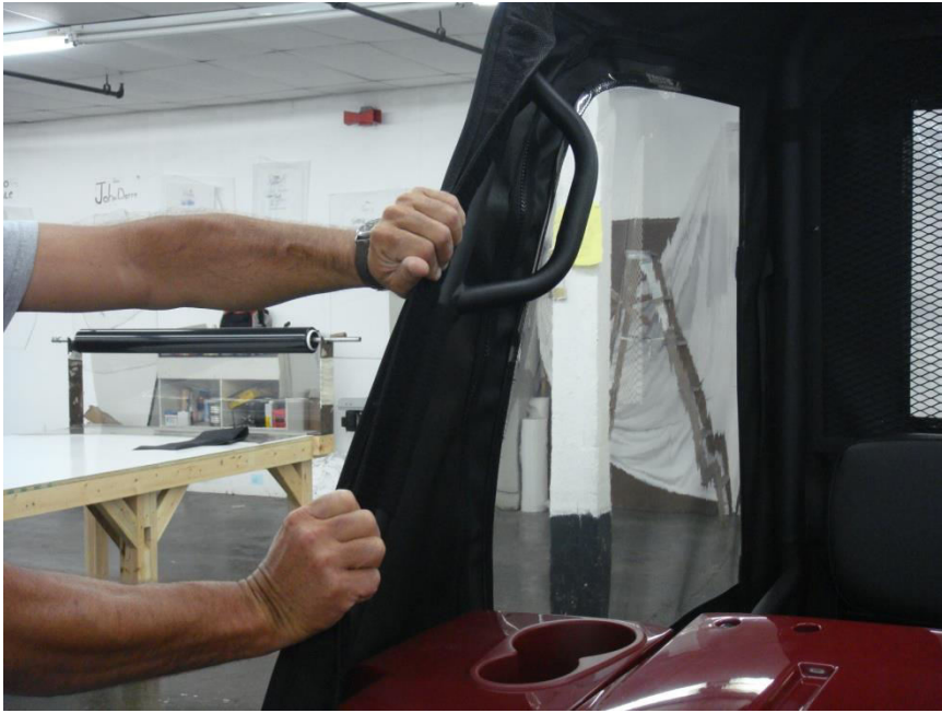
Figure 11.1 – attach Windshield Roll Bar post Velcro Tabs to installed 39” Velcro Strips
