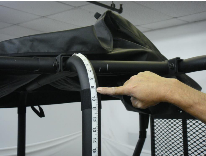
Figure 4.3 – install two 6" Velcro strips horizontally around the Center Roll Bar upright one @ 4" & one @ 9" below the cross-member weld
