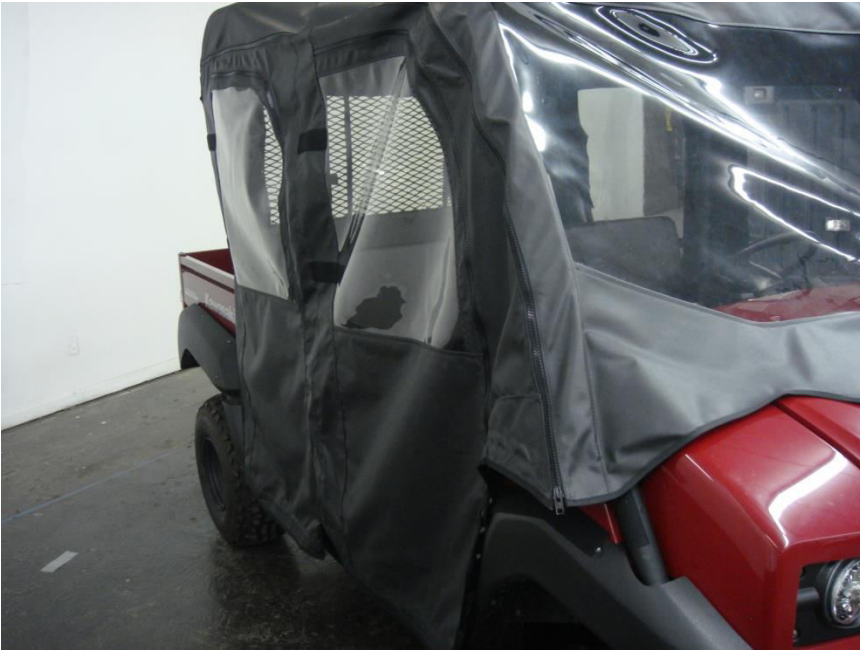
Figure 7.3 - align enclosure with all panels attached on the Roll Cab Frame so corner Enclosure seams are located near the center of the roll bars
