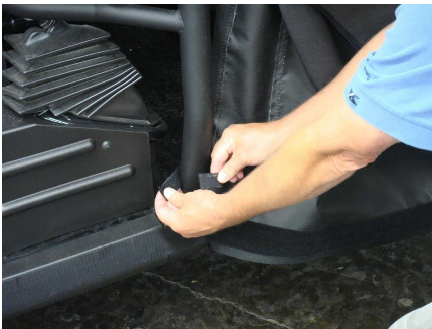
Figure 9.2 - attach 6" Rear Roll Bar Post enclosure Velcro tabs to the installed Velcro strips at the bottom of the Rear Roll Bar post upright
