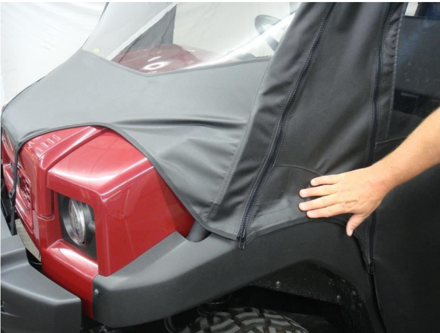
Figure 12.2 - attach Dash Cowl / Fender Well Side Velcro Tabs to installed Velcro strips
