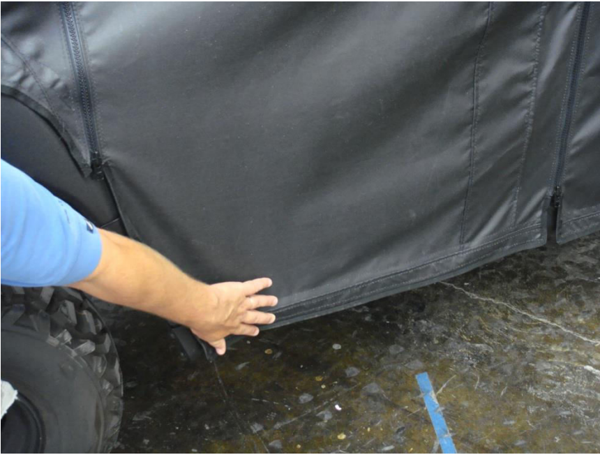
Figure 12.3 – attach front Rocker Panel Velcro tabs
