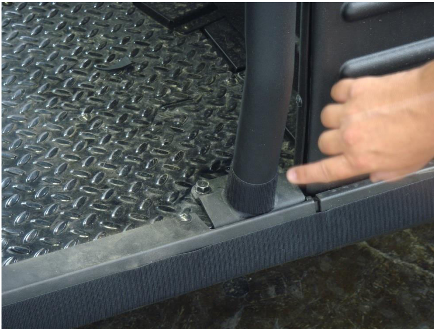
Figure 4.1 – install 6" Velcro Strip horizontally around the bottom of the Center Roll Bar upright
