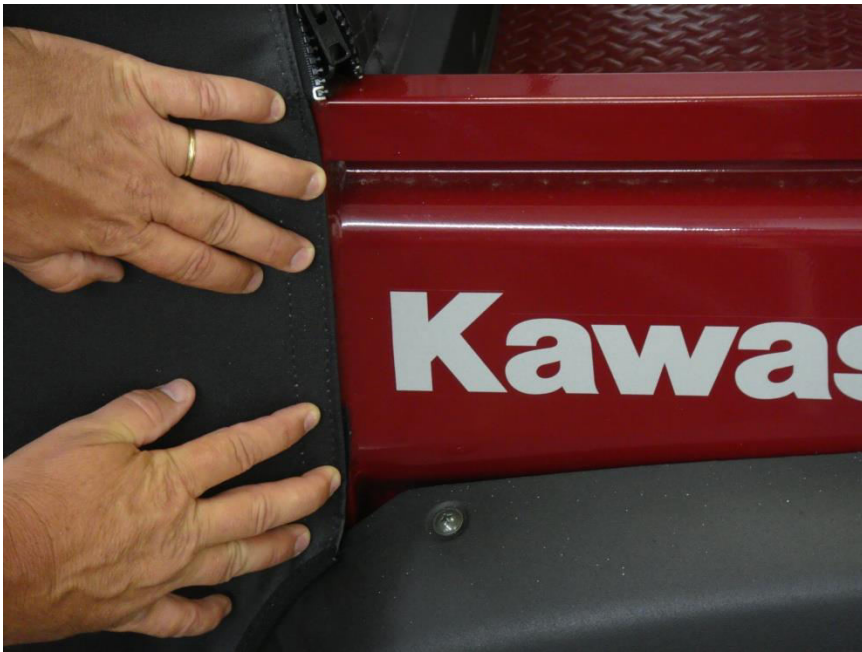
Figure 12.5 – attach 10” Velcro tabs to cargo bed
