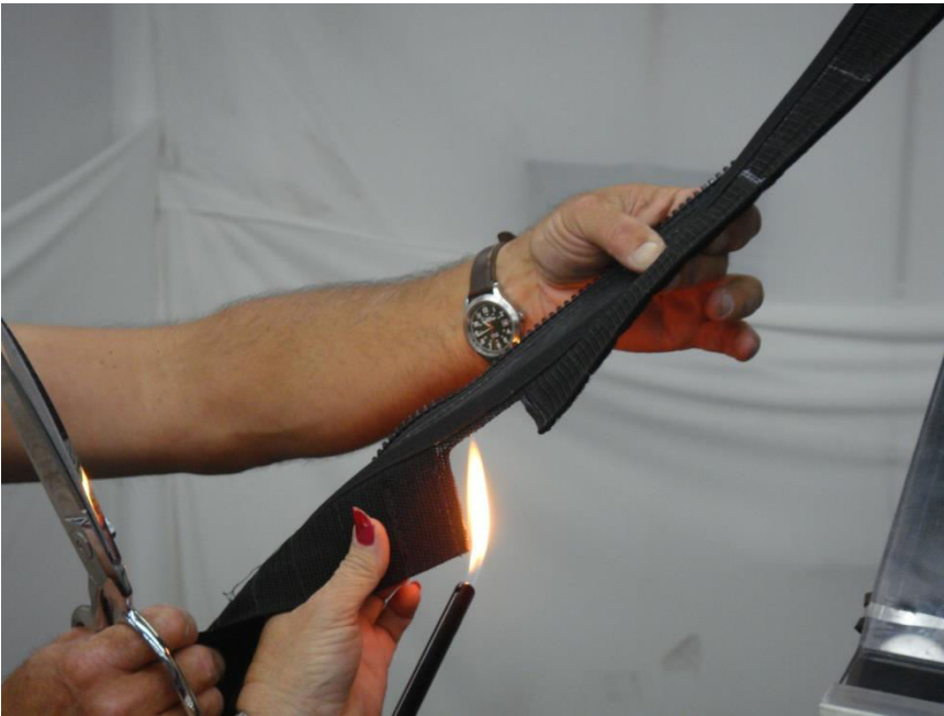
Figure 11.4 – Seal Frayed Tab thread at the cut area using a lighter
