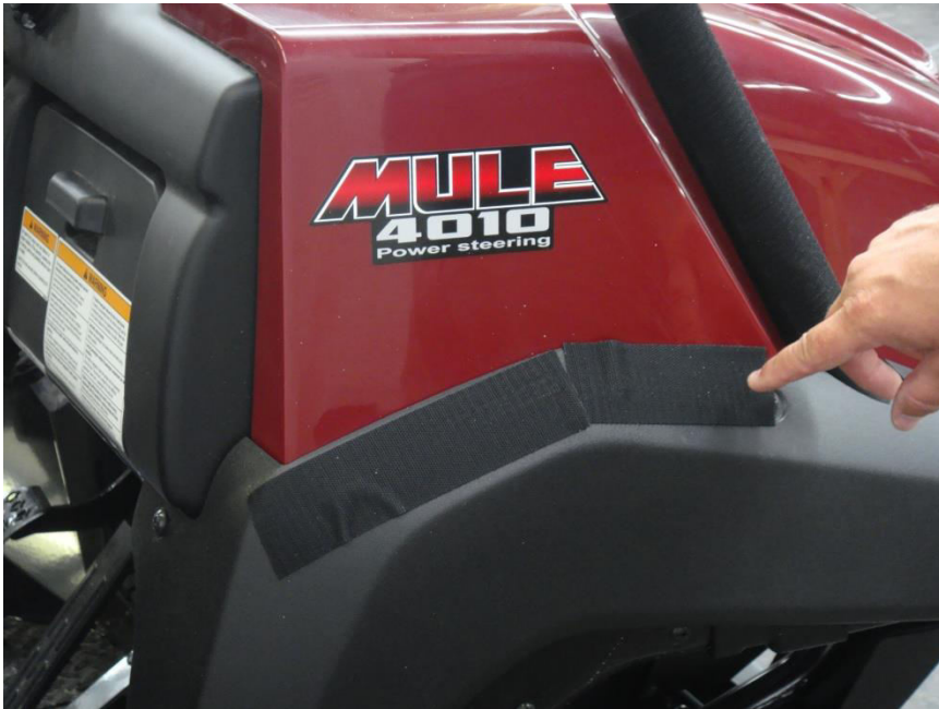
Figure 5.1 - Install the 13" Velcro Strips on the Dash Cowl / Fender Well – you will need to split the Velcro strip 8" X 5" before installing
