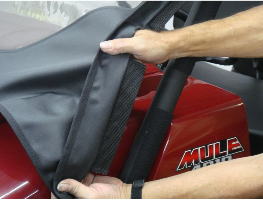
Figure 13.3 - attach bottom 8" Velcro Tabs to the installed Velcro Strips
