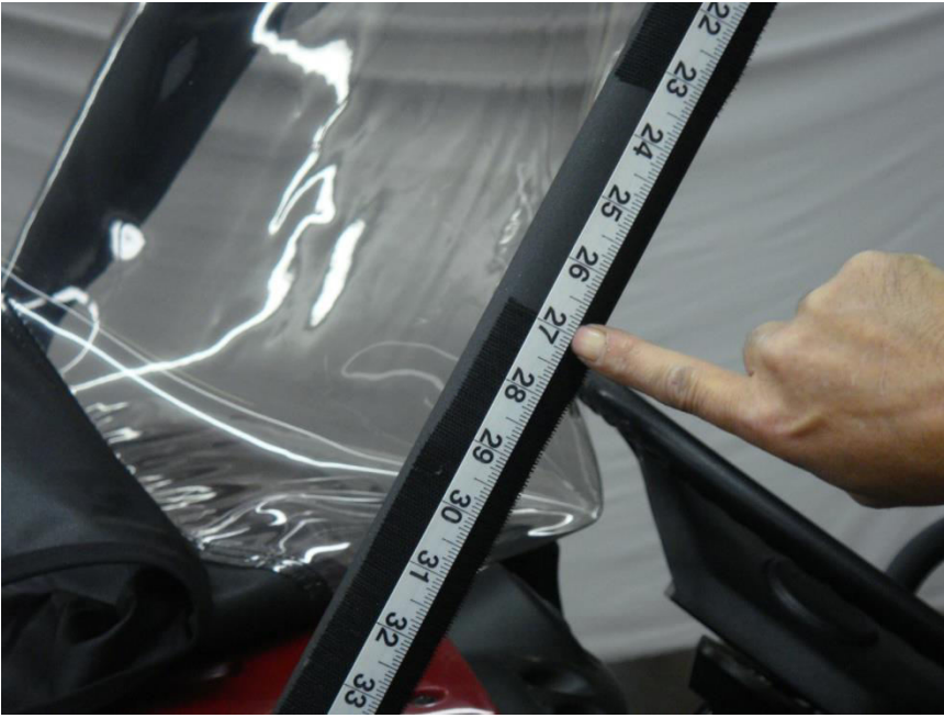
Figure 3.2 - install 8" Velcro Strip Vertically 27" below Roll Bar Cross-member weld joint
