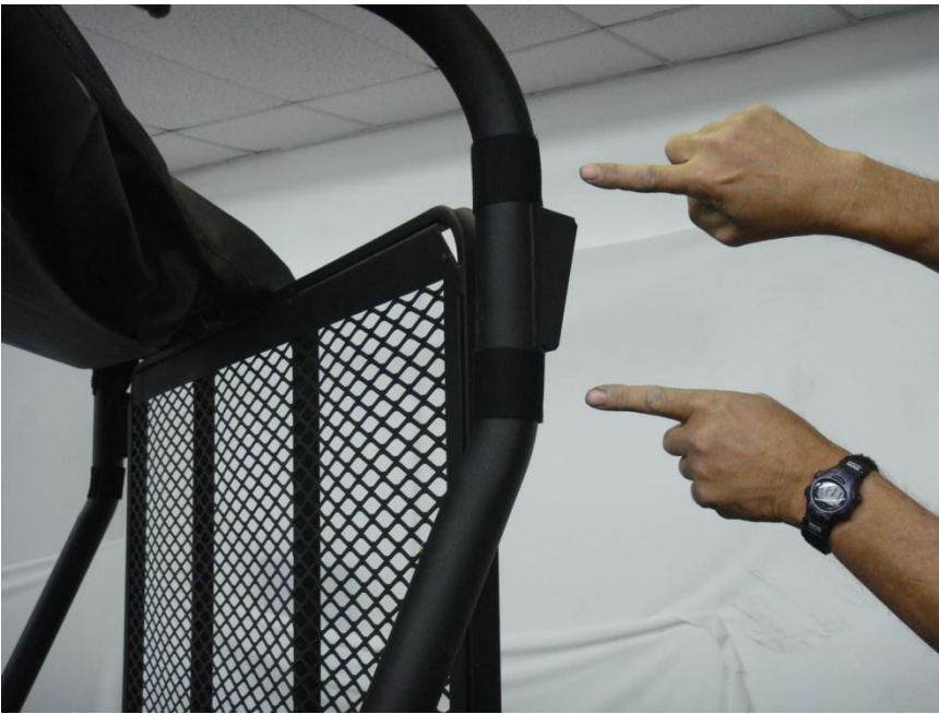
Figure 4.4 – install 6" Velcro strips horizontally at the top and bottom of the rear Roll Bar upright exhaust port
