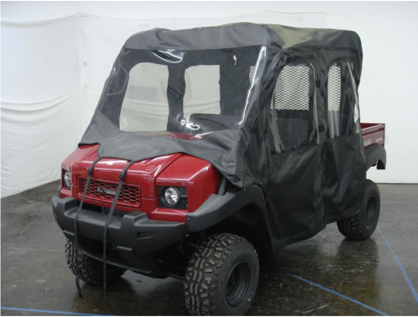
Figure 8.3 - align enclosure with all panels attached on the Roll Cab Frame so seams are located near the center of the roll bars
