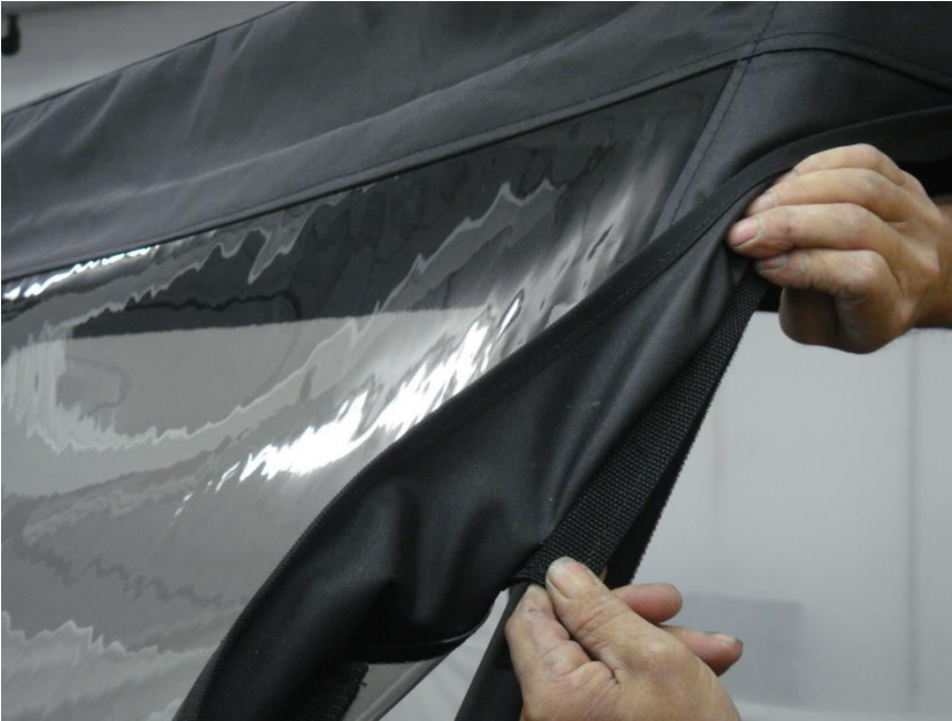
Figure 13.1 - attach top 8" Velcro Tabs to installed Velcro strips
