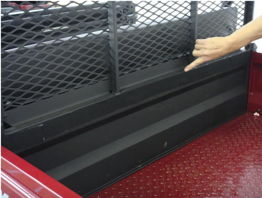
Figure 2.1 - install 46" Velcro Strip on Top Raised Panel below rear window
