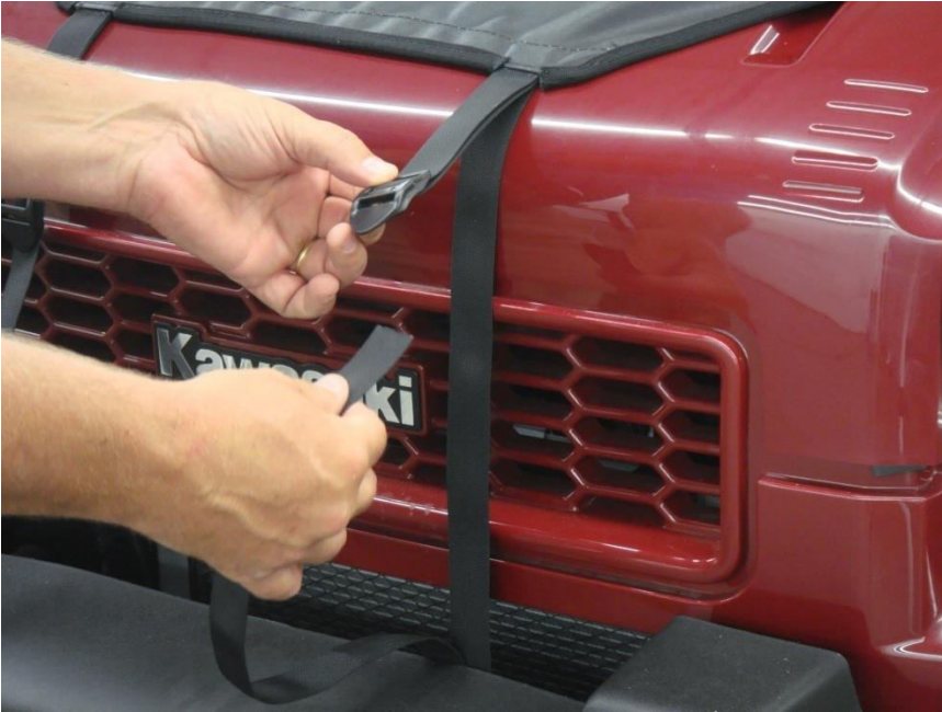
Figure 12.1 - Run Front Hood Straps around the Vehicle front bumper bar located behind the plastic Bumper Guard
