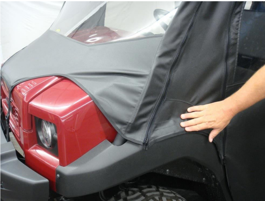
Figure 15.2 - attach Dash Cowl Side Velcro Tabs to installed Velcro strips
