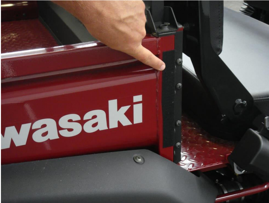
Figure 7.1 – install 10" (1" wide) Velcro Strips vertically to the Cargo Bed
