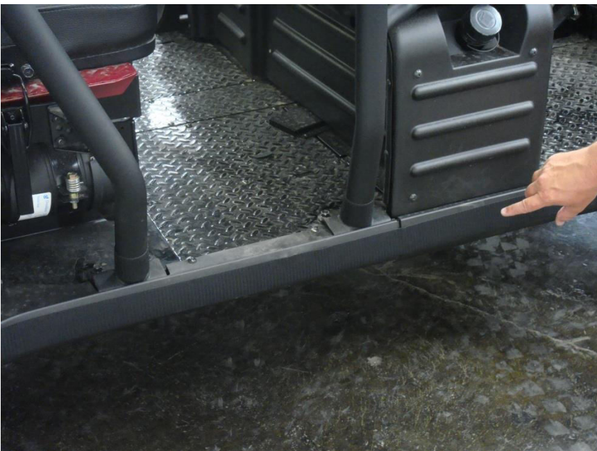
Figure 6.2 - install Rear Door Rocker Panel 25" Velcro Strip
