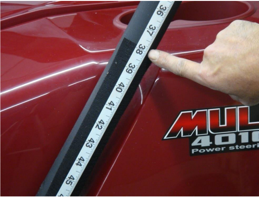
Figure 3.3 - install 8" Velcro strip Vertically 38" below Roll Bar Cross-member weld joint
