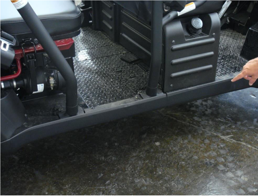
Figure 6.1 - install Front Door Rocker Panel 28" Velcro Strip
