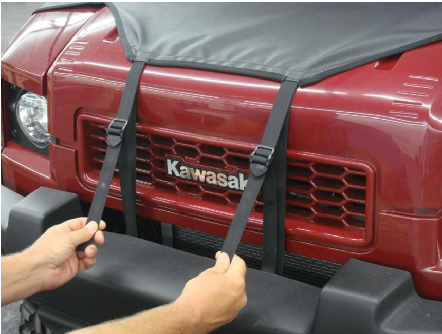
Figure 14.1 - tighten front hood straps until front windshields wrinkles are straightened out
