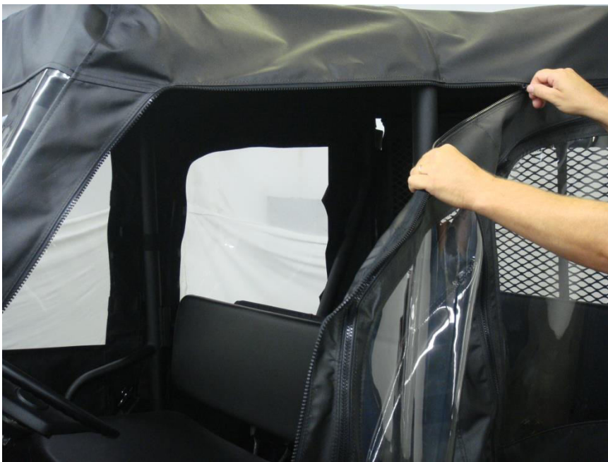
Figure 8.1 - Attach Door Panels by zipping them to the Top / Front Windshield panels
