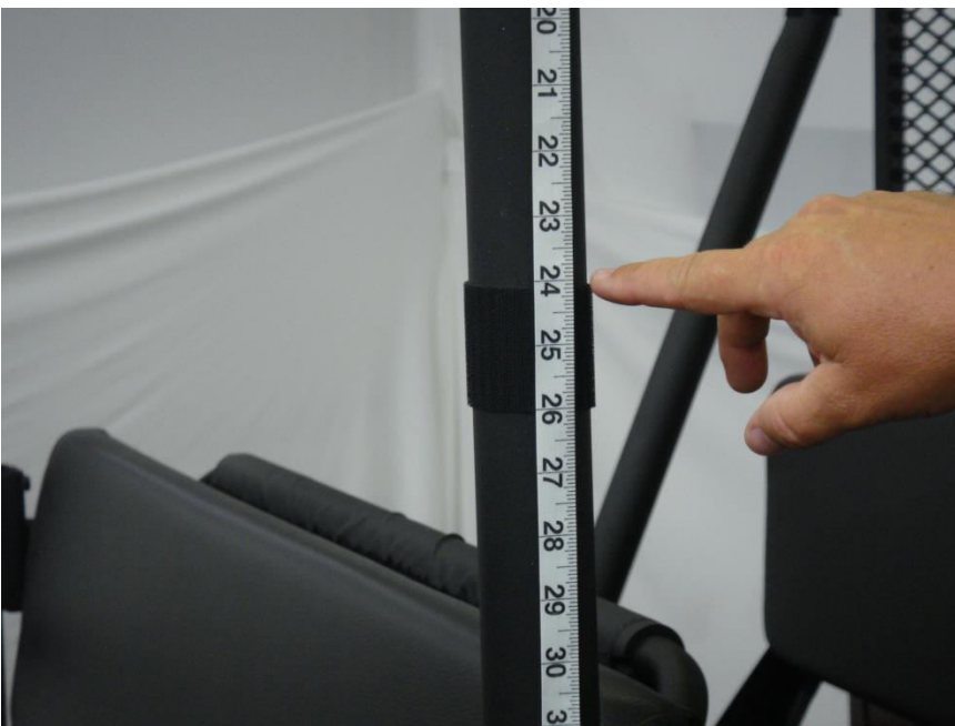
Figure 4.2 – install 6" Velcro Strip horizontally around the Center Roll Bar upright 24" below the cross-member weld joint
