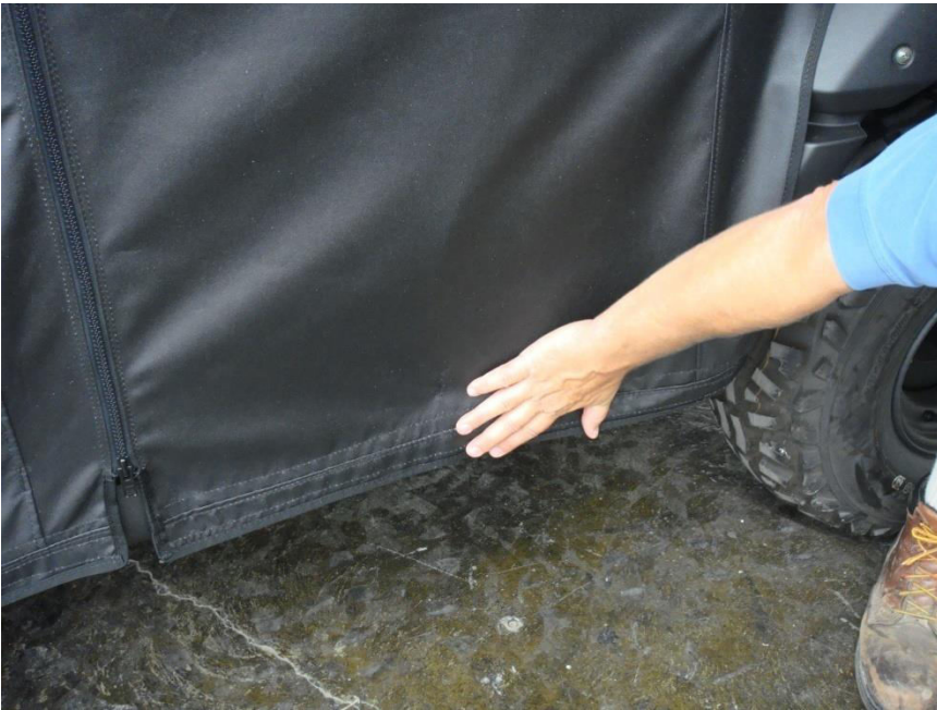
Figure 16.2 - attach Rear Door Rocker Panel Velcro Tabs
