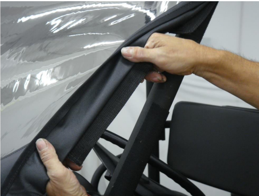
Figure 13.2 - attach center 8" Velcro Tabs to installed Velcro strips
