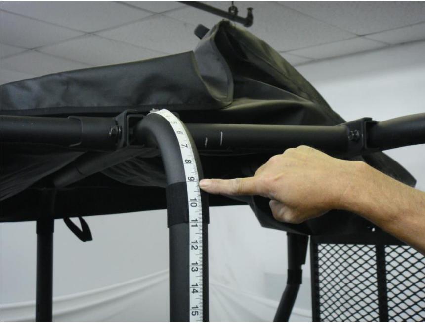
Figure 4.3 – install 6" Velcro strip horizontally around the Center Roll Bar upright 9" below the cross-member weld jointt
