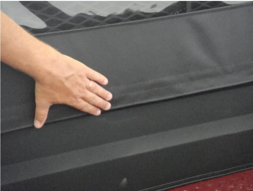
Figure 9.1 - square rear of enclosure to cab and attach rear enclosure Velcro tab to installed 46" Velcro strip
