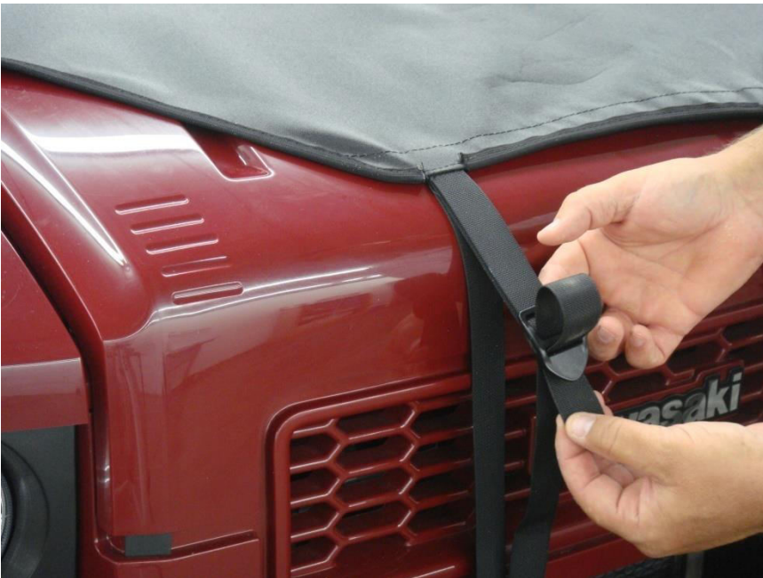
Figure 12.2 - Thread front Hood Strap into the buckles starting upward through the back of the buckle through the top opening
