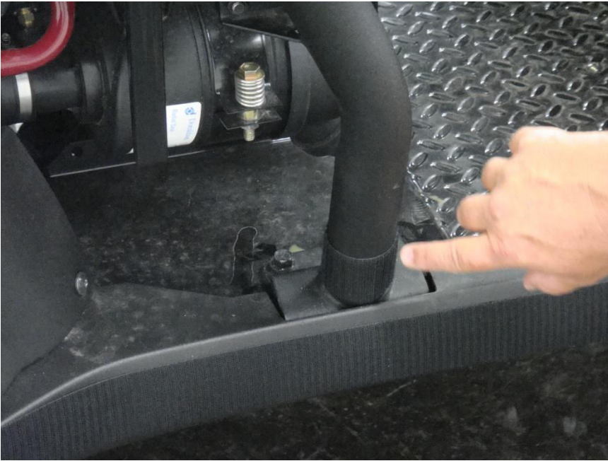
Figure 4.5 – install 6” Velcro Strip horizontally around the bottom of the Rear Roll Bar upright
