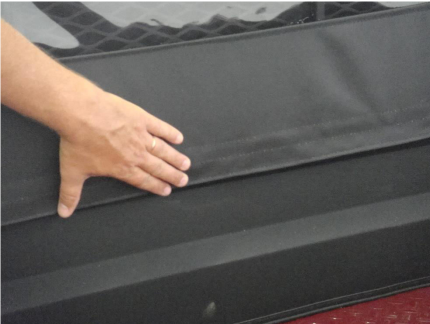
Figure 6.1 - square rear of enclosure to cab and attach rear enclosure Velcro tab to installed 47" Velcro strip
