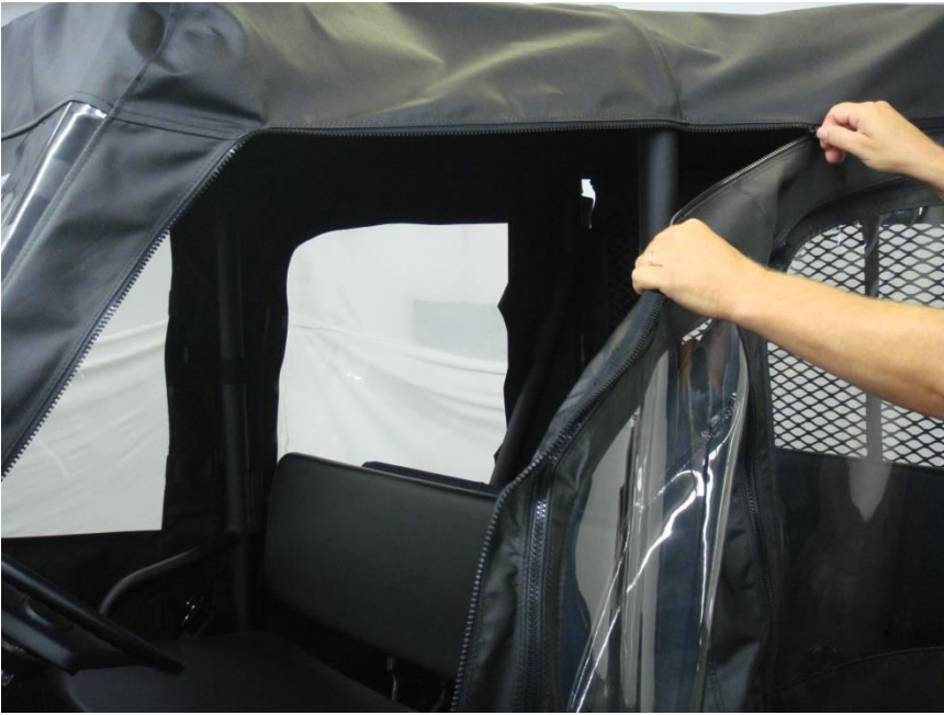
Figure 5.1 - Attach Door Panels by zipping them to the Top / Front Windshield panels
