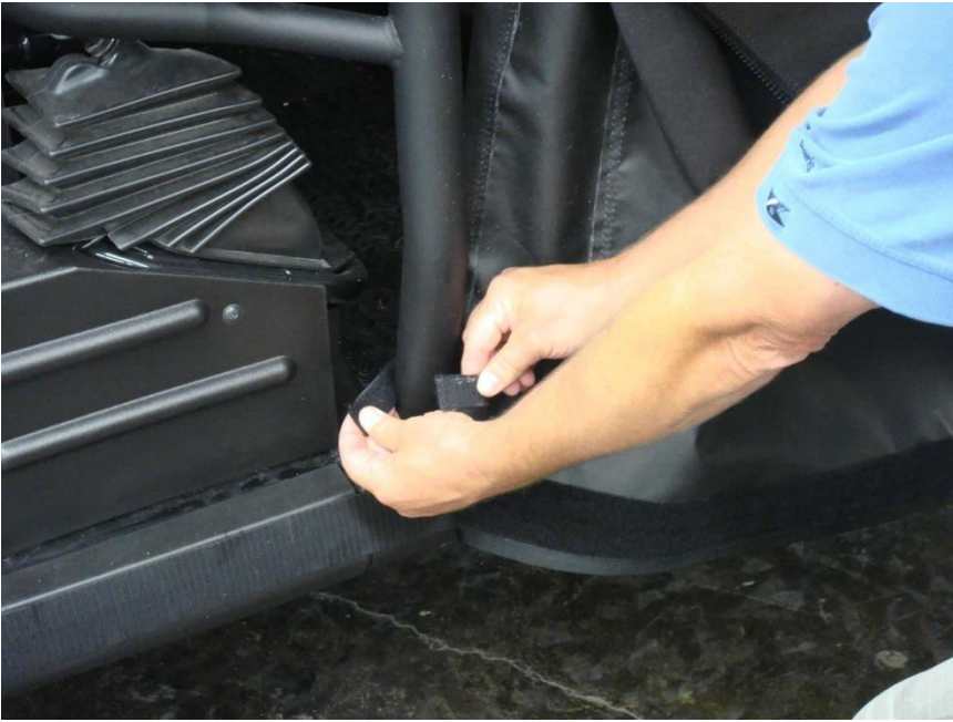
Figure 8.2 - attach Center Roll Bar upright enclosure bottom tabs to installed 6" Velcro strips
