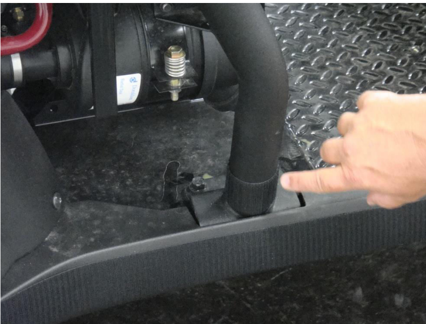
Install 6 1/2" Velcro Strip horizontally around the bottom of the Rear Roll Bar upright
