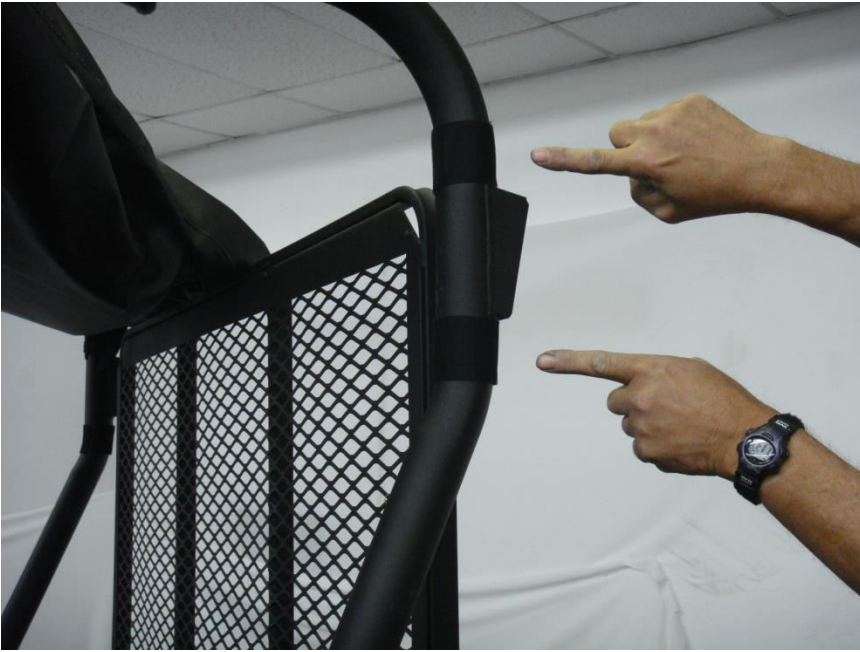
Install two 6" Velcro strips horizontally at the top and bottom of the rear Roll Bar upright exhaust port
