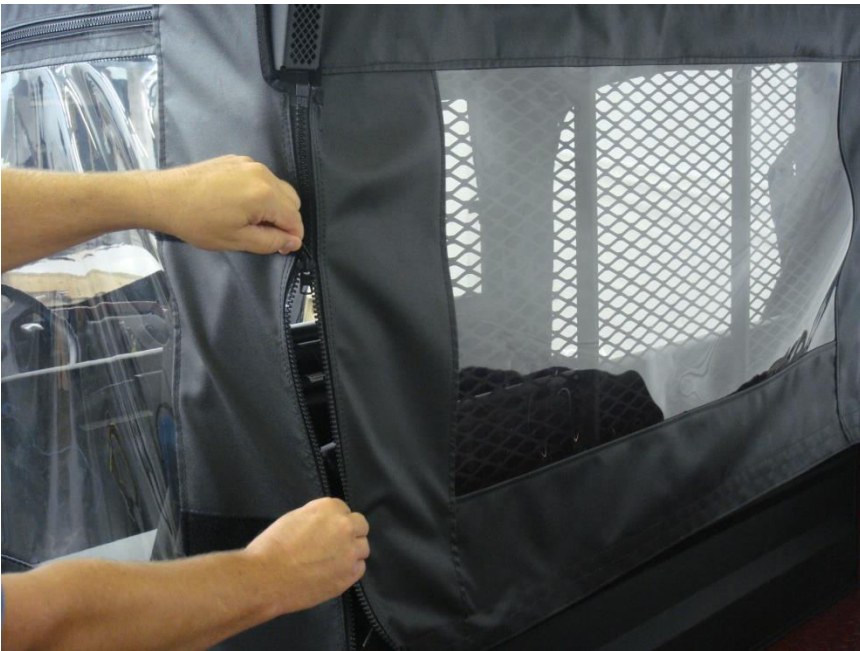
Figure 5.2A - attach Rear Window Panel by Zipping it to the Top and Door Panels. Note Rear Roll Bar Exhaust port must be exposed
