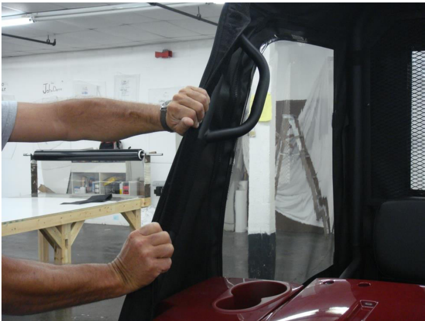
Figure 9.1 – attach Windshield Roll Bar post Velcro Tabs to installed 40" Velcro Strips
