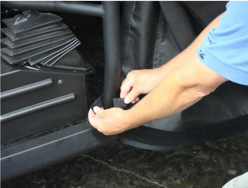
Figure 7.2 - attach Rear Roll Bar Post enclosure Velcro tabs to the installed Velcro strips at the bottom of the Rear Roll Bar post upright
