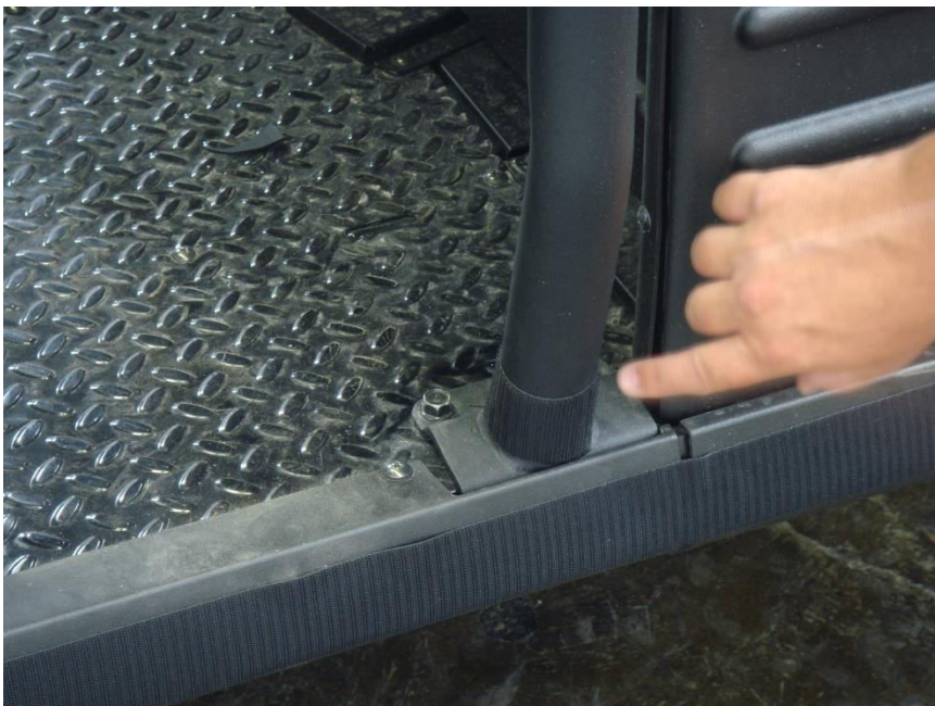
Install 6" Velcro Strip horizontally around the bottom of the Center Roll Bar upright
