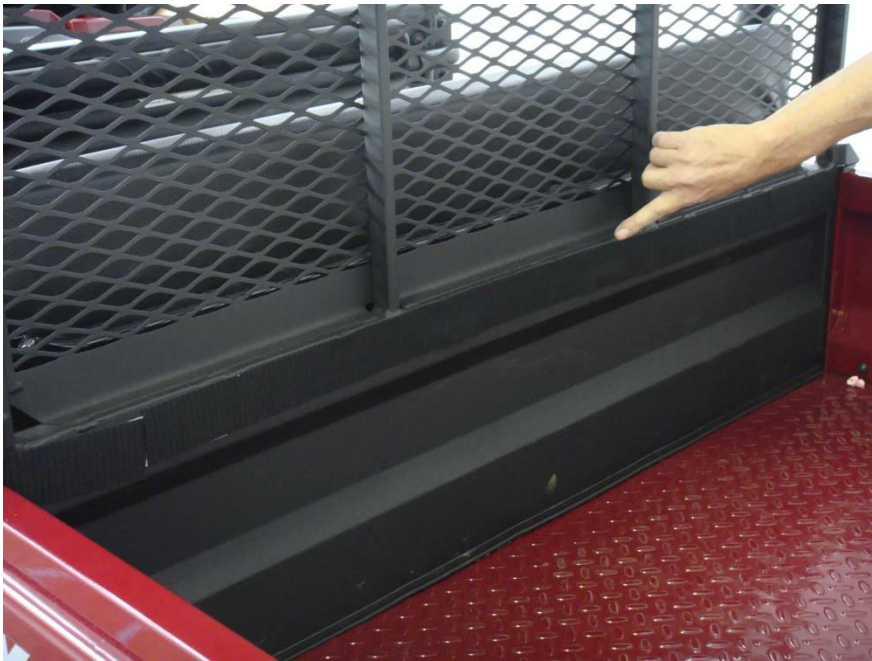
Install 46" Velcro Strip on Top Raised Panel below rear window
