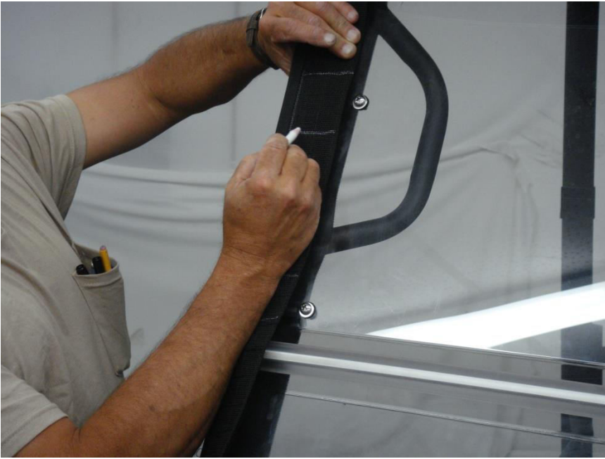
Figure 9.2 - Mark windshield tabs where hard windshield clamps are located along the windshield Roll Bar
