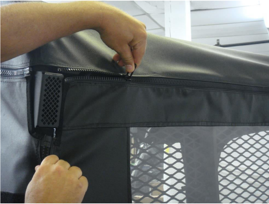
Figure 5.2B – attach Rear Window Panel by Zipping it to the Top and Door Panels. Note Rear Roll Bar Exhaust port must be exposed
