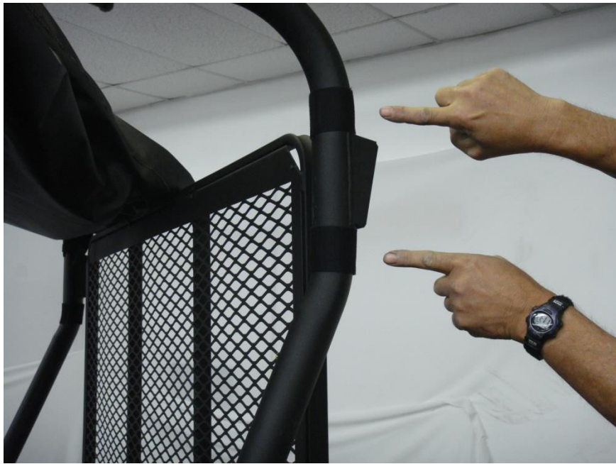
Adhesive hook reference D & E-Wrap adhesive hook strips horizontally around roll bar.
