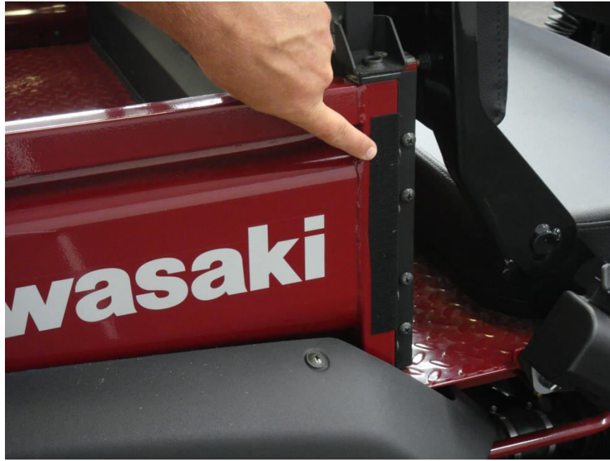
Adhesive hook reference G-Attach 1" adhesive hook strip vertically near front of cargo bed.
