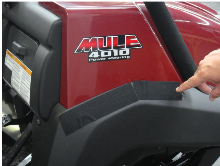
Adhesive hook reference N-Split 12" adhesive hook strip to curve corresponding to sewn in loop strips.
