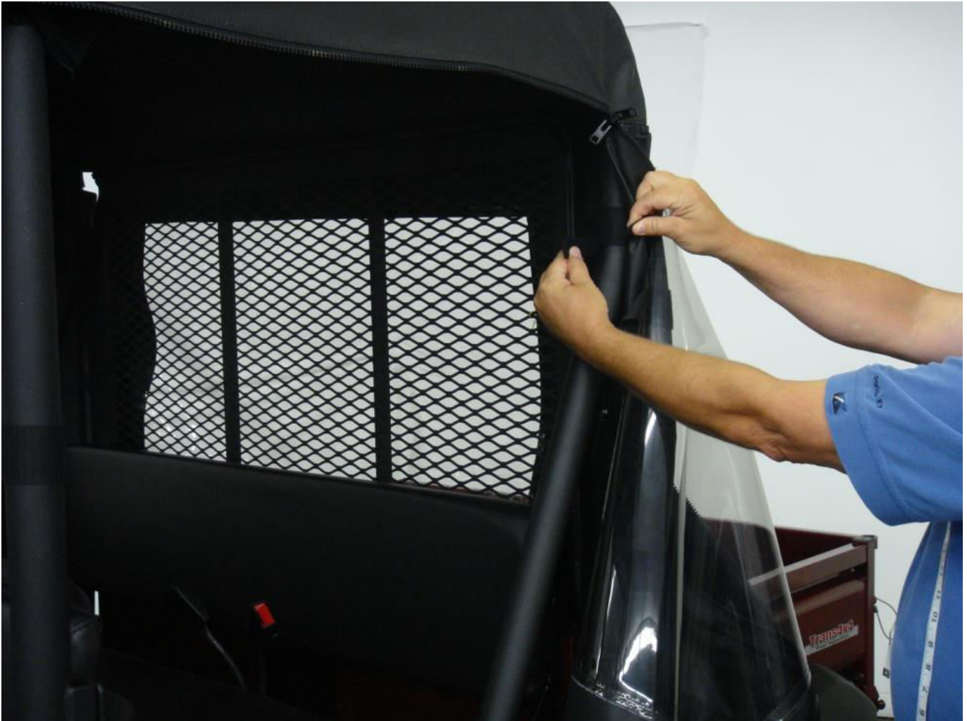
Figure 7.1 - Example of wrapping double-sided velcro strips around adhesive velcro.
