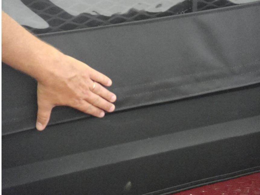
Figure 4.1 - square rear of enclosure to cab and attach rear enclosure Velcro tab to installed 46" Velcro strip
