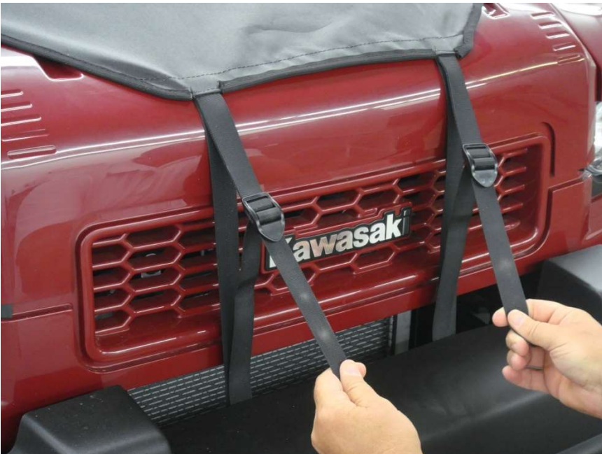
Figure 10.1 – fully tighten hood straps by pulling downward on both straps at the same time until front windshield is tight
