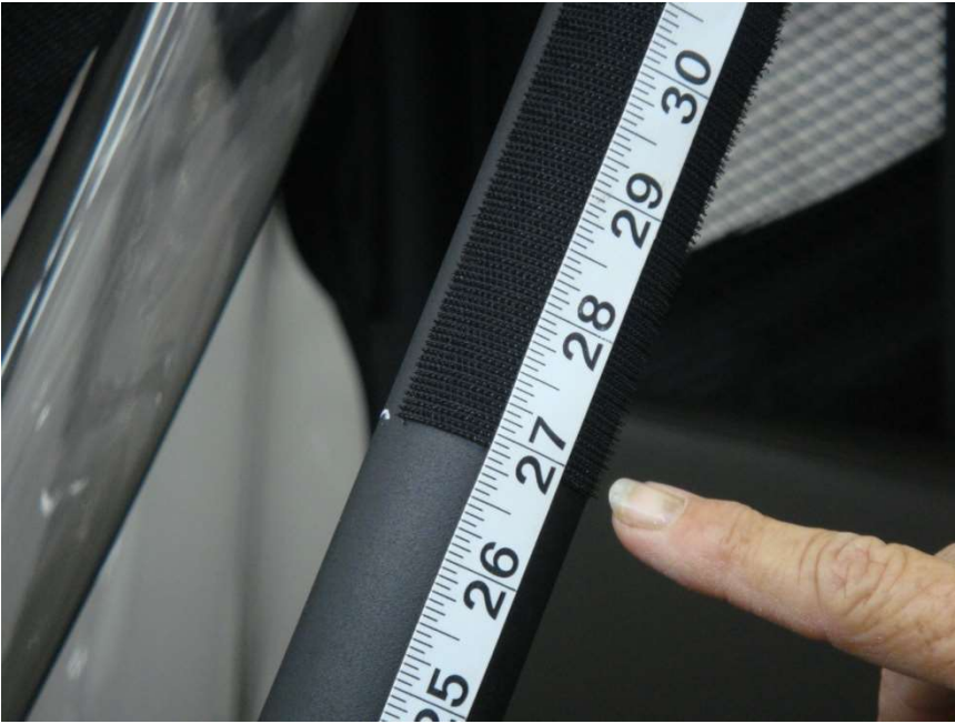
Figure 2.3 - 8" Velcro Strips placed vertically 27" above the front roll bar post bolts
