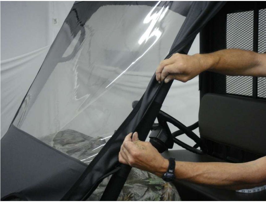
Figure 9.2 - attach middle front Roll Bar Velcro Tab pulling outward and downward toward the front of the vehicle
