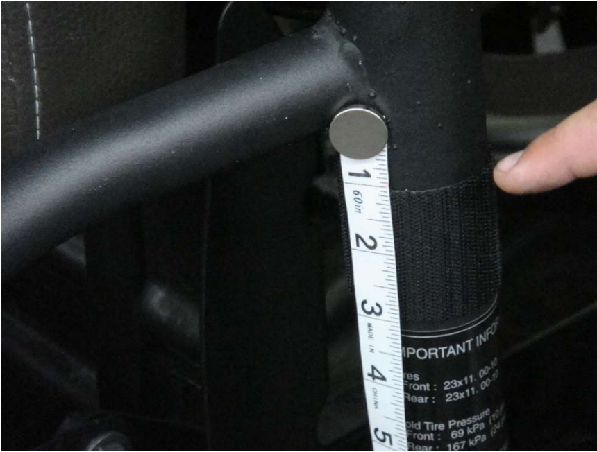
Figure 3.1 - 6" Velcro placed horizontally 1" below the Arm Rest Bar
