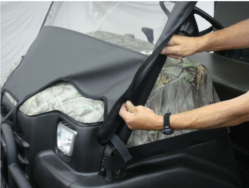
Figure 9.3 - attach lower front Roll Bar Velcro Tab pulling outward and downward toward the front of the vehicle
