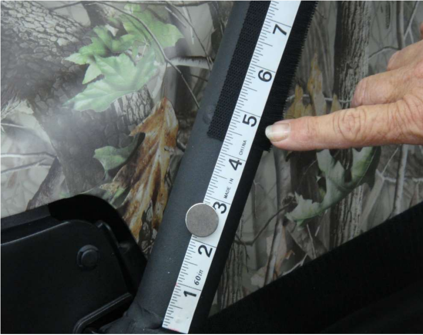
Figure 2.1 - 8" Velcro strips placed vertically 4 1/4" above the front roll bar post bolts
