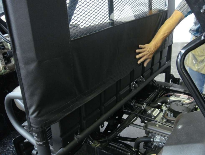
Figure 6.1 - square enclosure to frame and attach 49" rear cab Velcro tab to installed Velcro Strip
