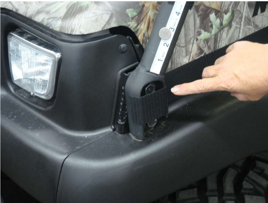
Figure 3.2 - 6" Velcro Strips placed Horizontally around the front Roll Bar Bolt Section
