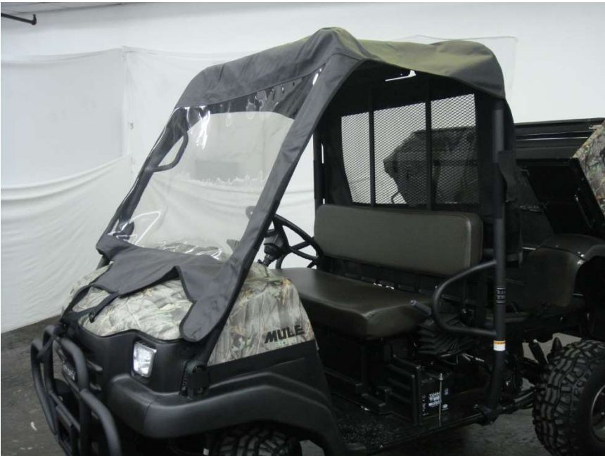
Figure 5.1 - place enclosure on vehicle cab roll bar structure
