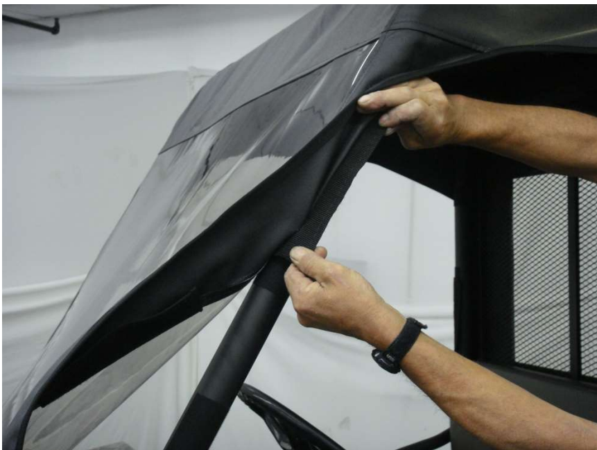
Figure 9.1 – attach top front Roll Bar Velcro Tab pulling outward and downward toward the front of the vehicle
