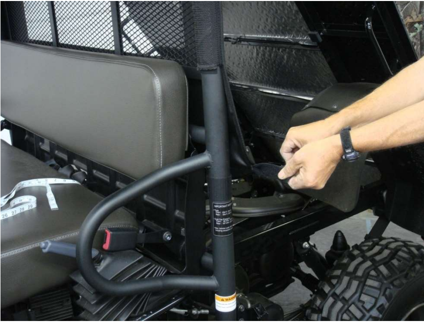
Figure 7.2 - attach Rear Roll Bar Post Velcro Tabs around Roll Bar just below the armrest
