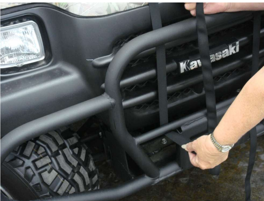
Figure 8.1 - run front hood straps through the center bar of the front bumper
