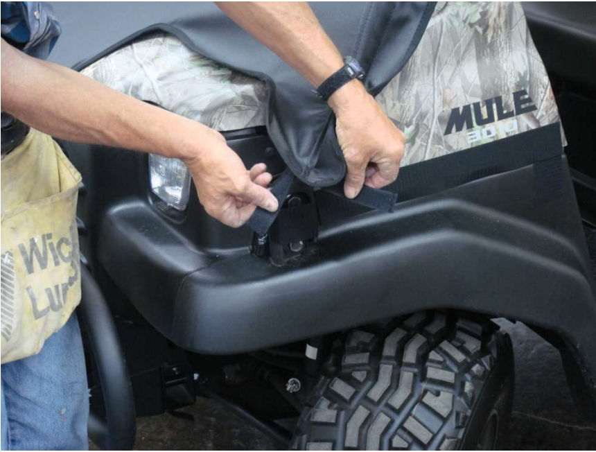
Figure 9.4 - attach bottom front Roll Bar Bolt section Velcro Tab horizontally around Roll Bar bolt section of the Roll Bar
