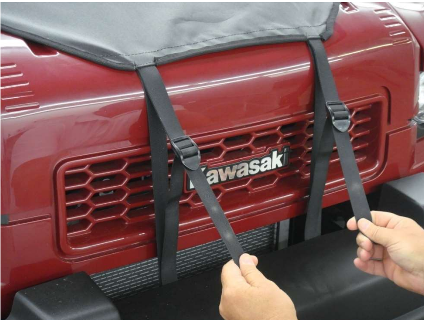
Figure 8.1 – fully tighten hood straps by pulling downward on both straps at the same time until front windshield is tight
