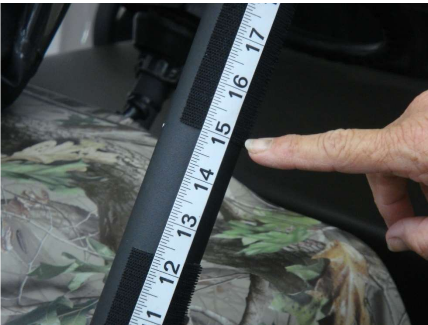
Figure 2.2 - 8" Velcro strips placed vertically 15" above the front roll bar post bolts
