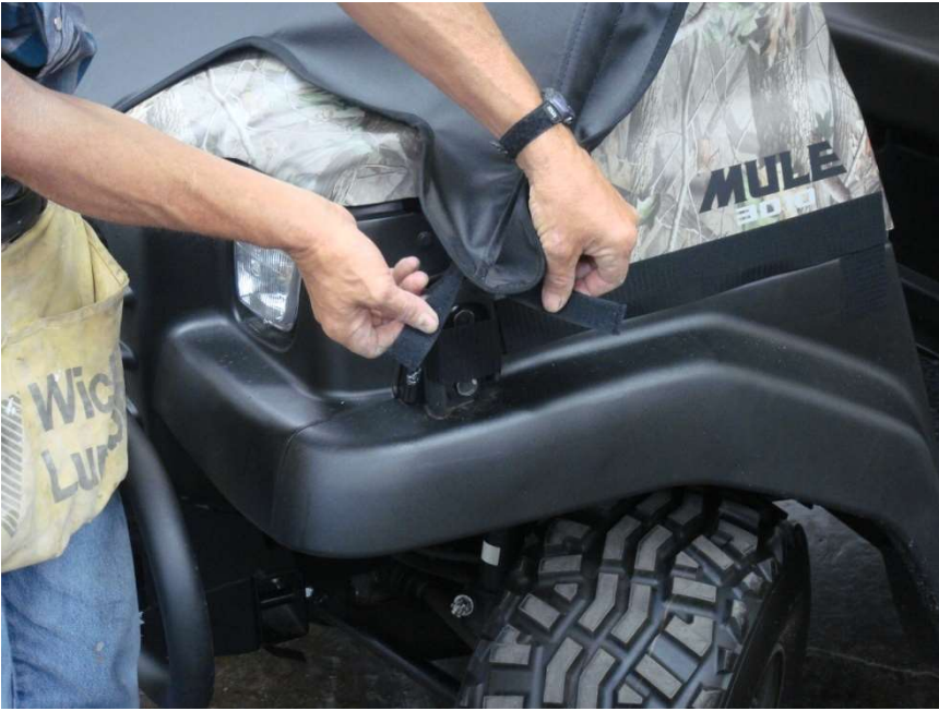
Figure 7.4 - attach bottom front Roll Bar Bolt section Velcro Tab horizontally around Roll Bar bolt section of the Roll Bar
