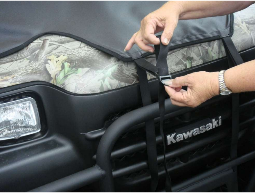
Figure 6.2 - thread front hood straps into buckles
