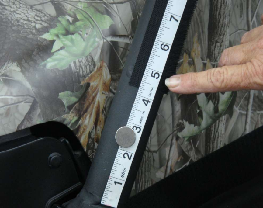
Figure 2.1 - 8" Velcro strips placed vertically 4 ¼" above the front roll bar post bolts
