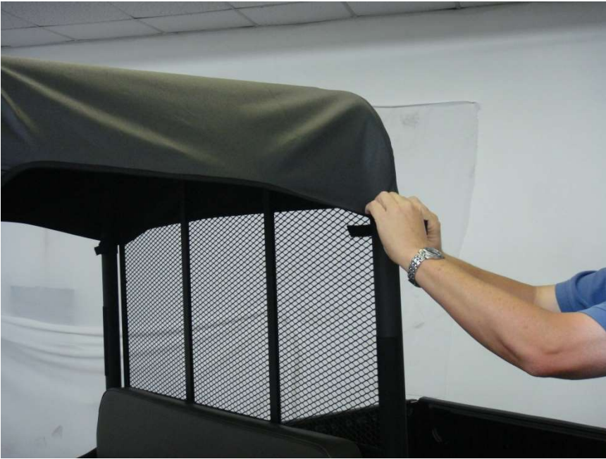
Figure 5.1 - attach Rear Roll Bar Post Velcro Tabs around installed Rear Roll Bar Velcro strips
