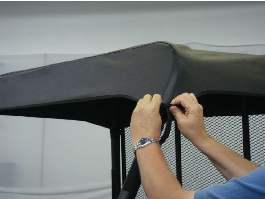
Figure 5.2 - Pull down firmly and attach front Velcro Tabs to installed Velcro strips
