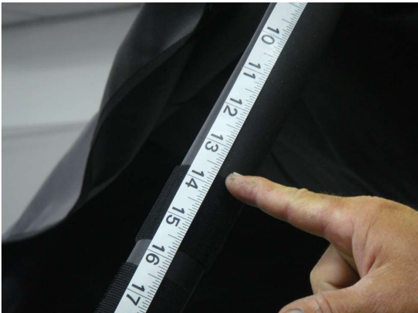
Figure 2.1 - place front Velcro strips horizontally around the front roll bar posts 13 ¾" below the roll bar cross member bracket located at the top of the cab roll bar structure.
