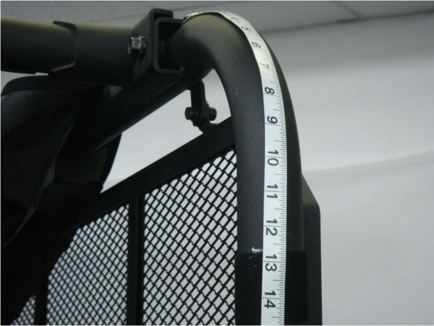
Figure 3.1 – Place Rear Velcro strips 12 ¾" inches below the top roll bar cross member brackets located at the top of the Cab Roll Bar Structure
