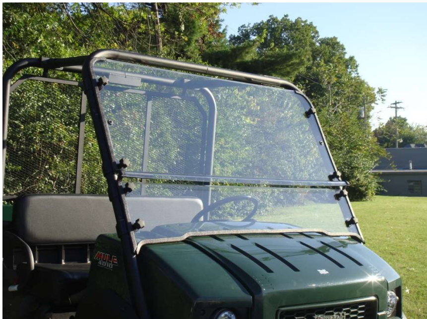
Figure 7.1 - Remove windshield plastic protective paper
