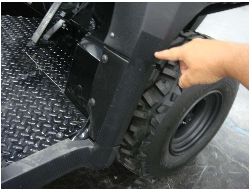
Figure 5.2 – 14 ½” Velcro strips placed vertically at the Front Lower Door Frame Area
