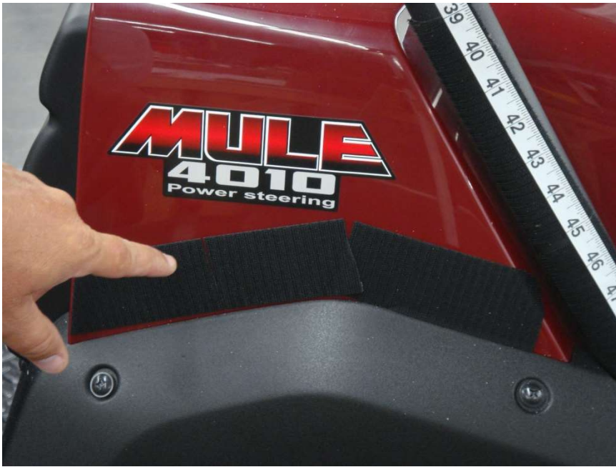
Figure 5.1 - 12” Velcro Strips placed horizontally on the side of the Dash Cowl – split to 8” and 4” sections
