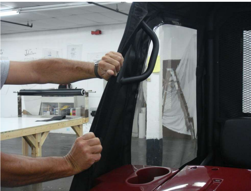
Figure 10.1 – attach Windshield Roll Bar Post Velcro Tabs to installed 36" Velcro Strips
