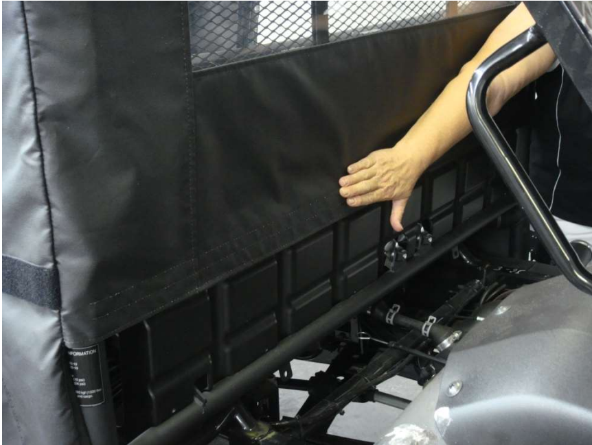
Figure 8.1 - square rear of enclosure to cab and attach rear enclosure Velcro tab to installed Velcro strip
