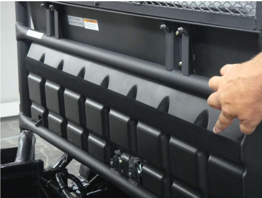
Figure 6.1 - 49” Velcro Strip Placed on the cab rear guard on the top raised rib
