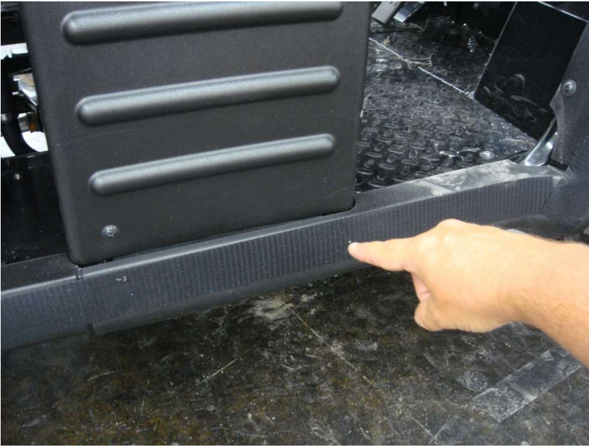
Figure 5.3 – 31” Velcro Strips placed along the Door Rocker Panel
