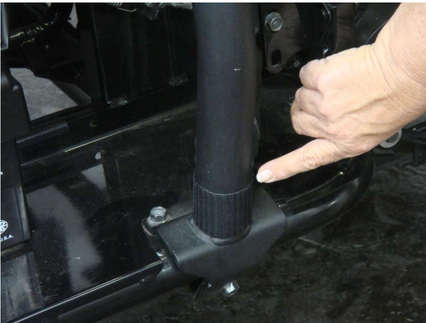
Figure 4.1 - 6" Velcro Strips placed horizontally at the base of the rear roll bar posts
