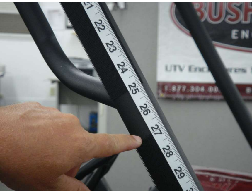
Figure 2.2 - 8" Velcro strips placed vertically 27" below the top roll bar cross member bolted section
