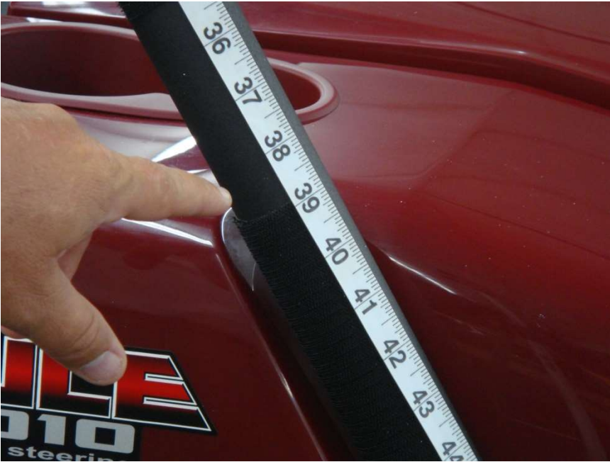
Figure 2.1 - 8" Velcro strips placed vertically 39" below the top roll bar cross member bolted section
