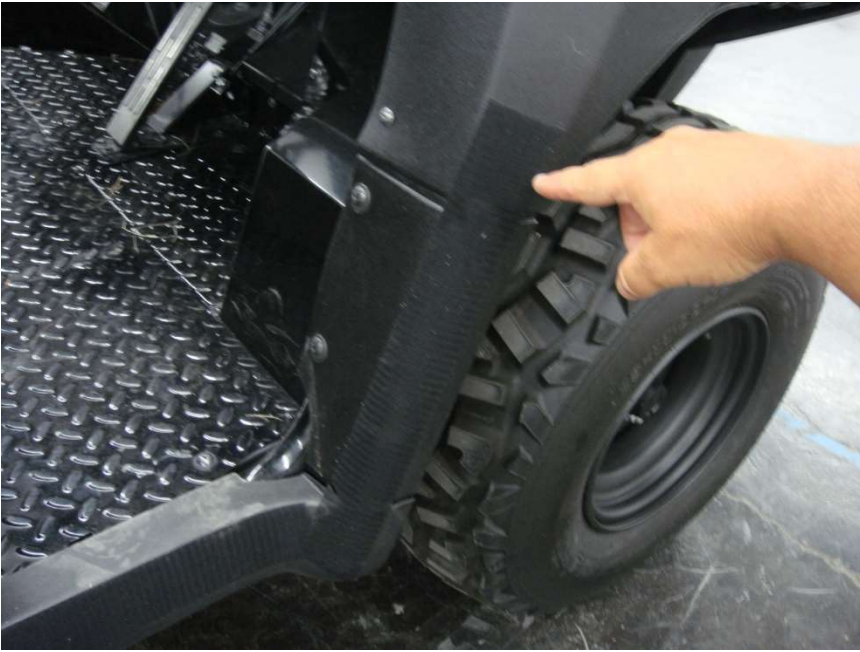
Figure 4.2 – 14 ½” Velcro strips placed vertically at the Front Lower Door Frame Area
