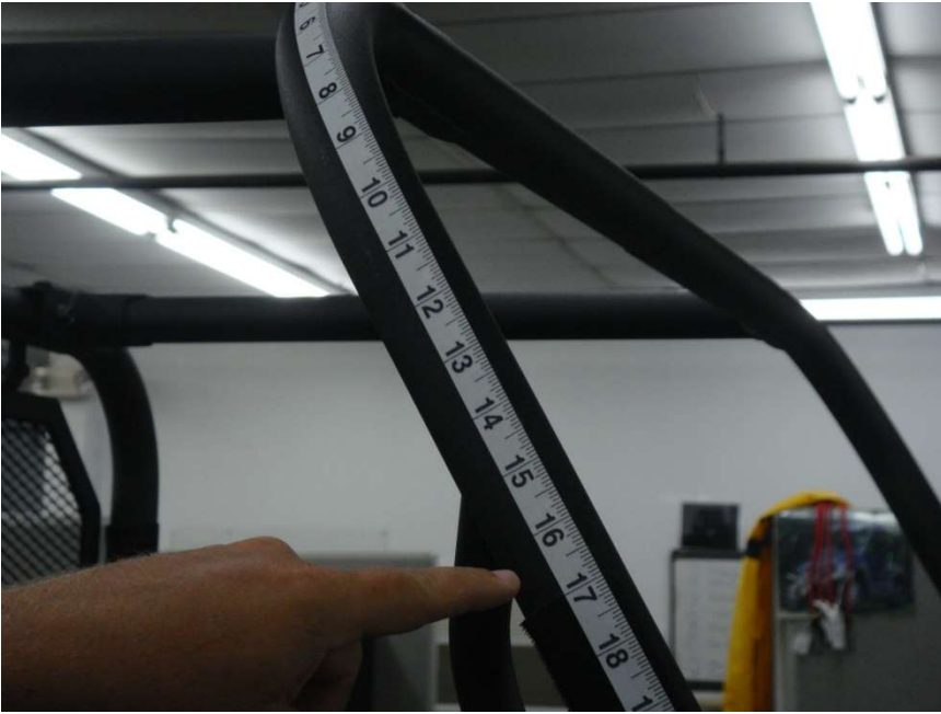
Figure 2.3 - 8" Velcro Strips placed vertically 17" below the top roll bar cross member bolted section
