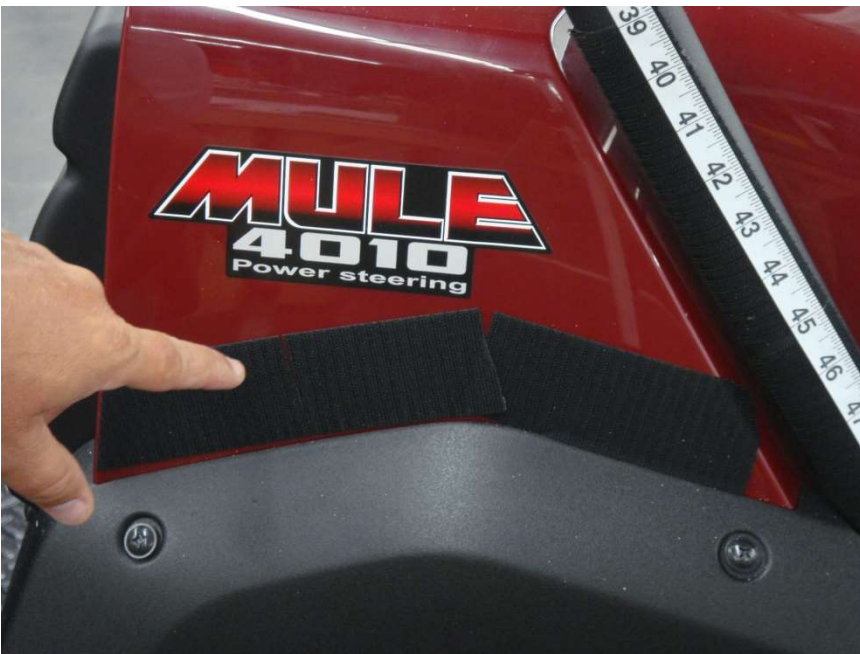
Figure 4.1 - 12" Velcro Strips placed horizontally on the side of the Dash Cowl – split to 8" and 4" sections
