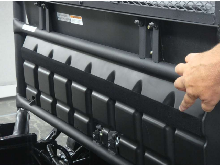
Figure 5.1 - 49" Velcro Strip Placed on the cab rear guard on the top raised rib
