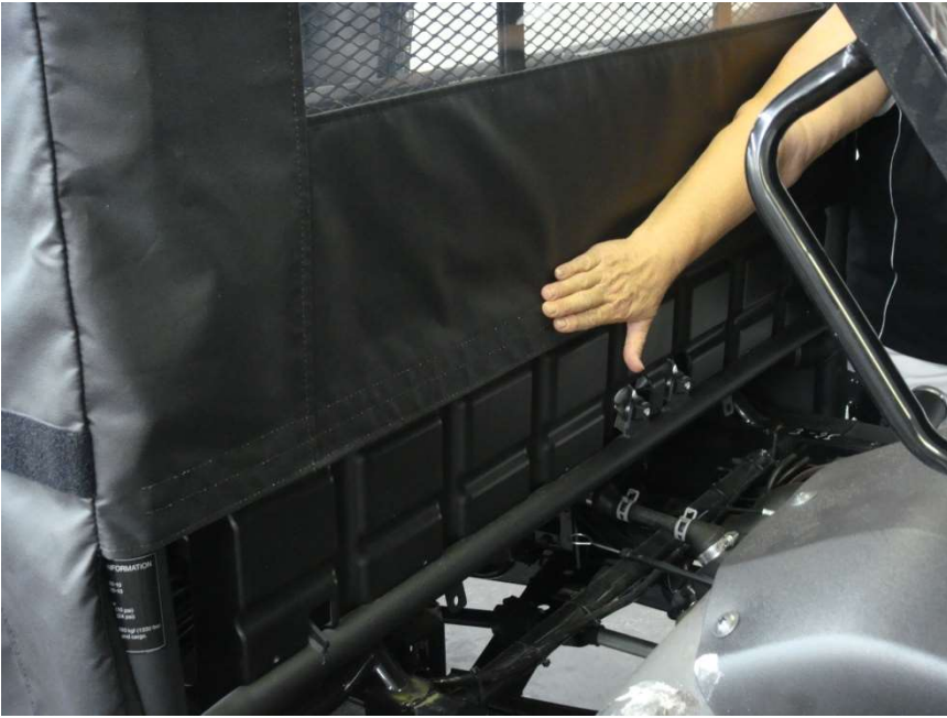
Figure 7.1 - square rear of enclosure to cab and attach rear enclosure Velcro tab to installed Velcro strip
