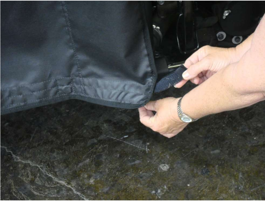
Figure 8.2 - attach Rear Roll Bar Velcro tabs at base of rear Roll Bar Posts
