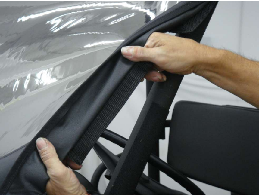
Figure 8.2 - attach middle front Roll Bar Velcro Tab pulling outward and downward toward the front of the vehicle
