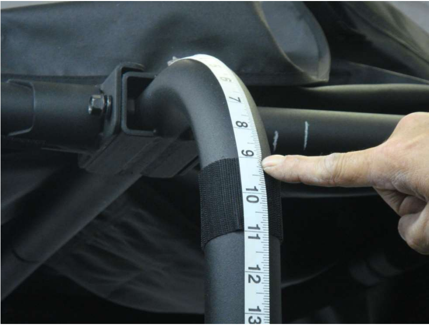
Figure 4.1 - install 6" Velcro strips horizontally 9" below top Roll Bar cross-member connecting bracket
