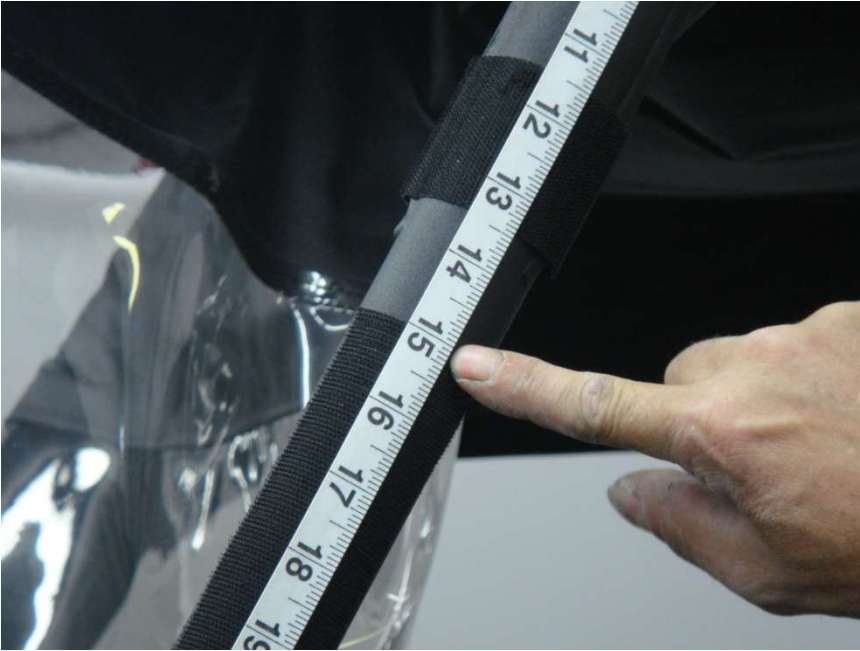
Figure 2.1 - 8" Velcro strips placed vertically 15" below the top Roll Bar cross-member weld joint
