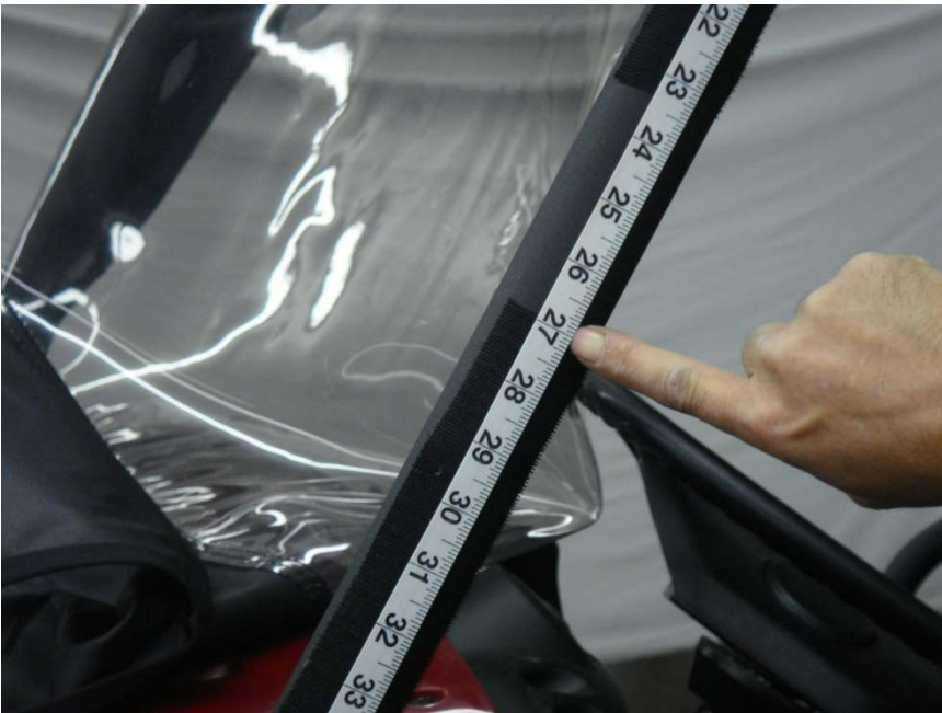
Figure 2.2 - 8" Velcro Strips placed vertically 27" below the top Roll Bar Cross-member weld joint
