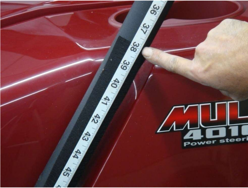
Figure 2.3 - install 8" Velcro Strip vertically 38" below the top Roll Bar Cross-member weld joint
