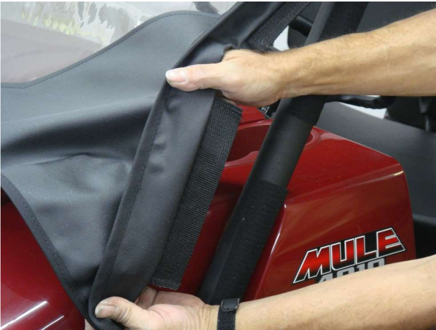
Figure 8.3 - attach lower front Roll Bar Velcro Tab pulling outward and downward toward the front of the vehicle
