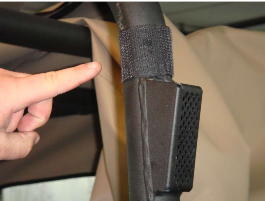
Figure 3.1 – place 6" Velcro strips horizontally around the rear Roll Bar post uprights just above the exhaust port
