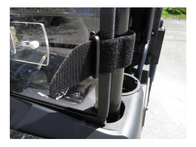
**Step 6:** Repeat Step 4 for each of the strap slots in the upper windshield section.
