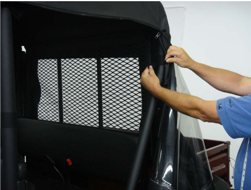
Figure 9.1 - attach 6 1/2" Rear Roll Bar post enclosure Velcro tabs to installed Velcro strips above and below the Roll bar exhaust port
