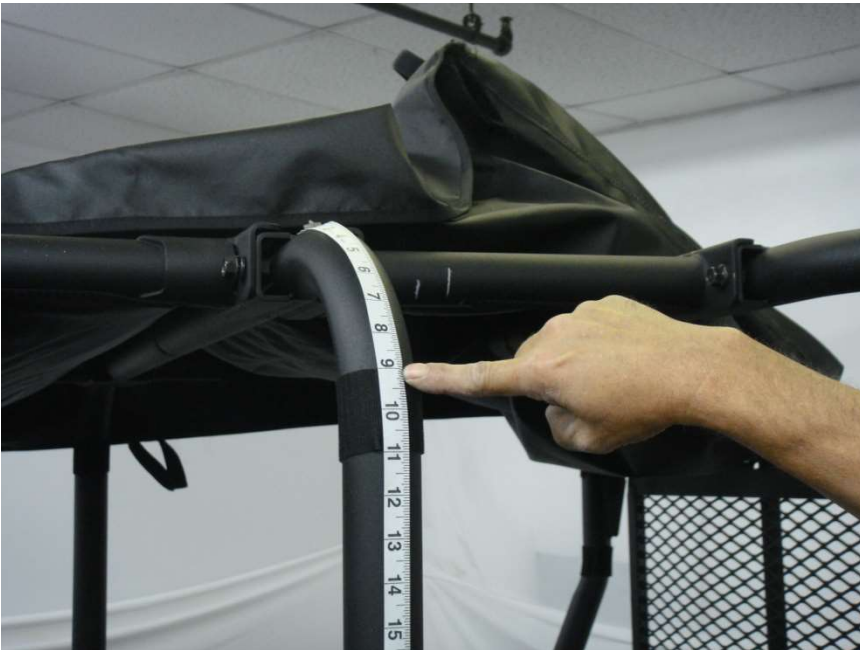
Figure 4.3 – install two 6 1/2" Velcro strips horizontally around the Center Roll Bar upright one @ 4" & one @ 9" below the cross-member weld
