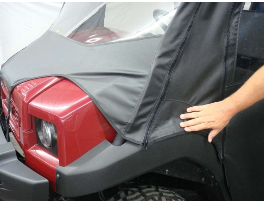
Figure 12.1 - attach Dash Cowl / Fender Well Side Velcro Tabs to installed Velcro strips
