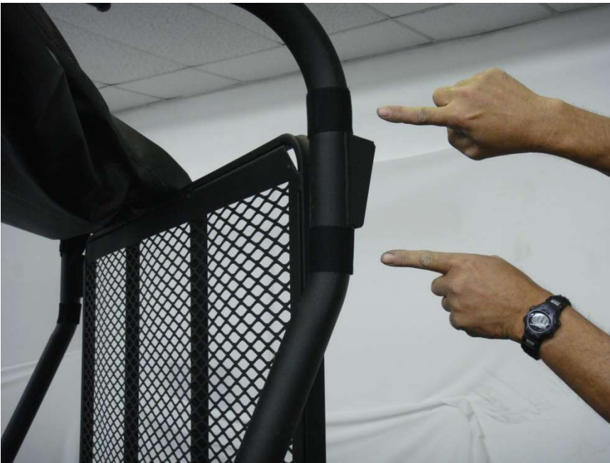
Figure 4.4 – install two 6" Velcro strips horizontally at the top and bottom of the rear Roll Bar upright exhaust port
