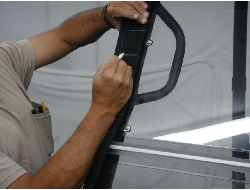
Figure 11.2 - Mark windshield tabs where hard windshield clamps are located along the windshield Roll Bar
