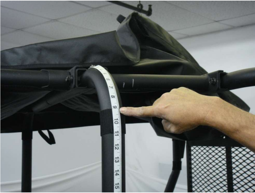
Figure 4.3 – install 6" Velcro strips horizontally around the Center Roll Bar upright approx 8" below the cross-member weld
