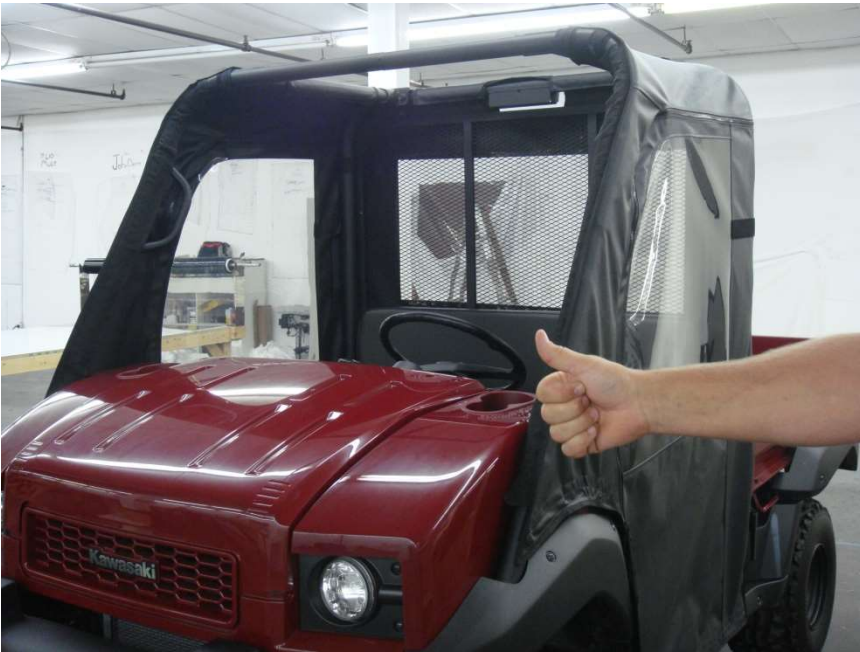
Figure 13.1 - follow steps 9 through 12 tightening Velcro and straps until enclosure is fully tightened to the Cab structure
