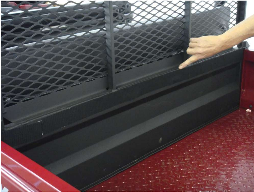
Figure 2.1 - install 47" Velcro Strip on Top Raised Panel below rear window
