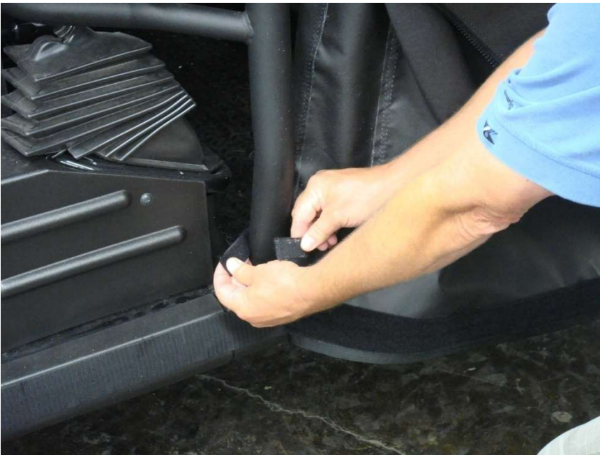
Figure 9.2 - attach 6 1/2" Rear Roll Bar Post enclosure Velcro tabs to the installed Velcro strips at the bottom of the Rear Roll Bar post upright
