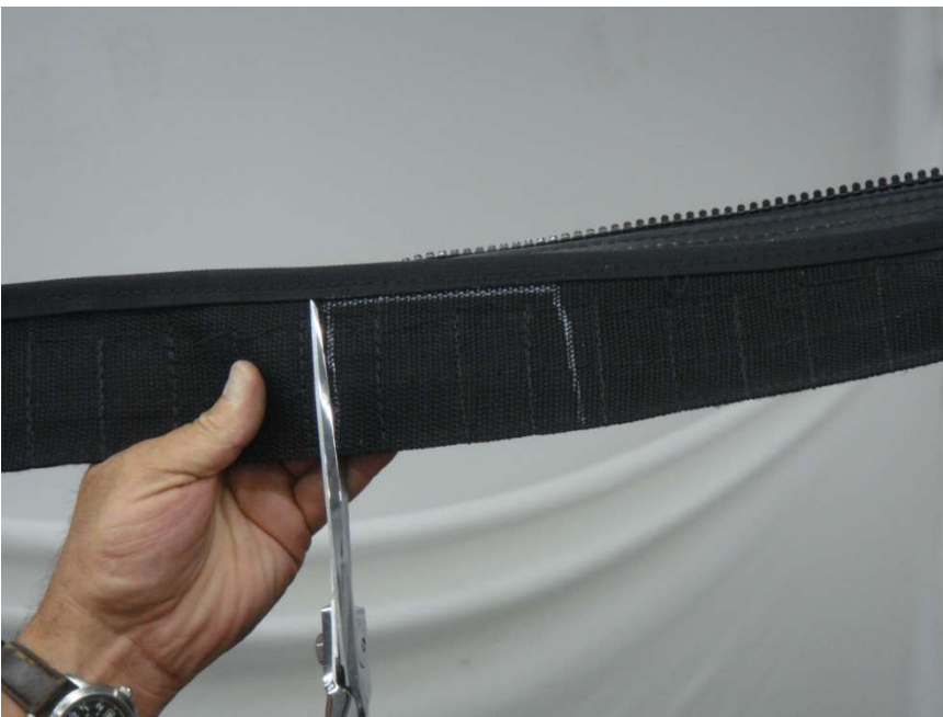
Figure 11.3 – Cut the Tab being very careful not to cut the binding at the edge
