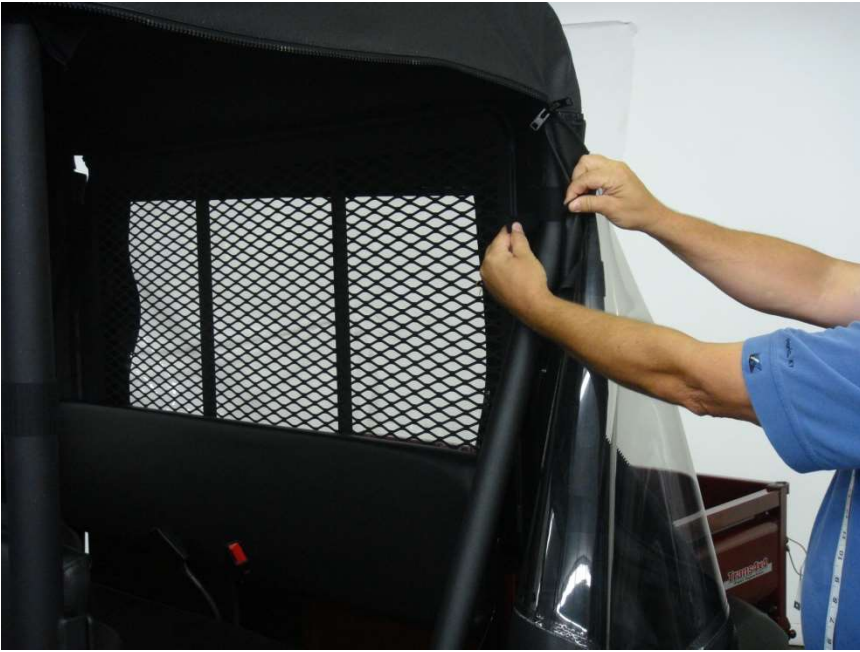
Figure 9.1 - attach 6 " Rear Roll Bar post enclosure Velcro tabs to installed Velcro strips above and below the Roll bar exhaust port
