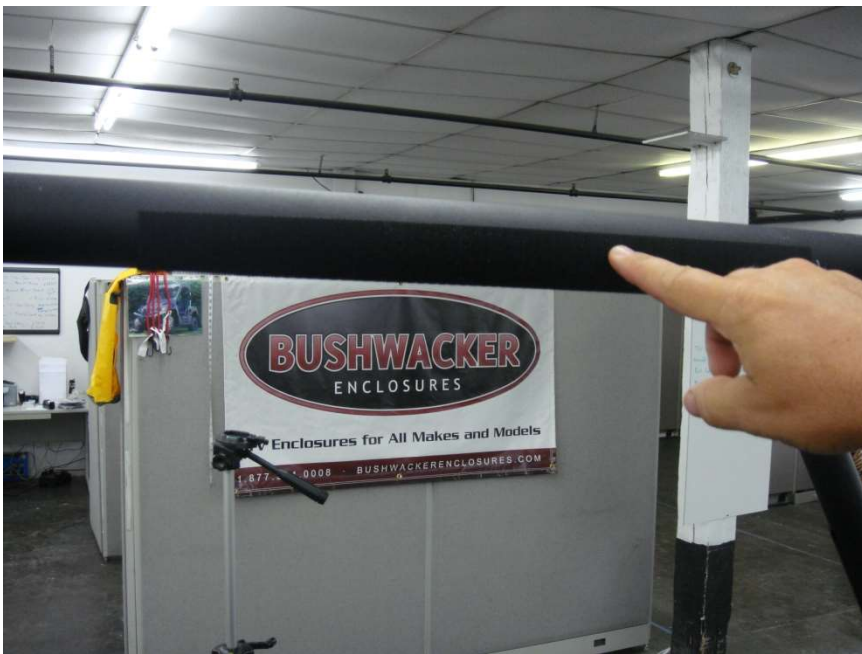
Figure 6.2 – install 4 ½", 17 ½", 7", 5", and 13" Velcro strips to top Roll Bar Cross members
