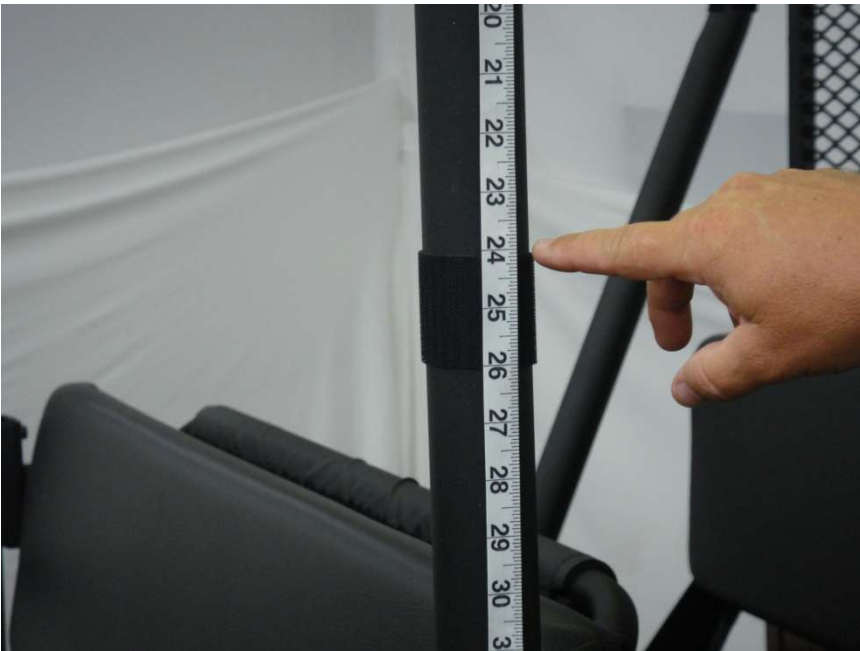
Figure 4.2 – install 6" Velcro Strip horizontally around the Center Roll Bar upright approx 24" below the cross-member weld joint
