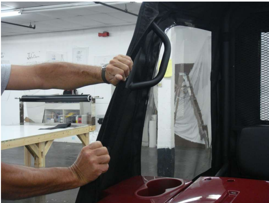
Figure 11.1 – attach Windshield Roll Bar post Velcro Tabs to installed 40" Velcro Strips
