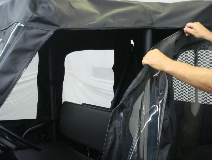
Figure 7.1 - Attach Door Panels by zipping them to the Top / Front Windshield panels
