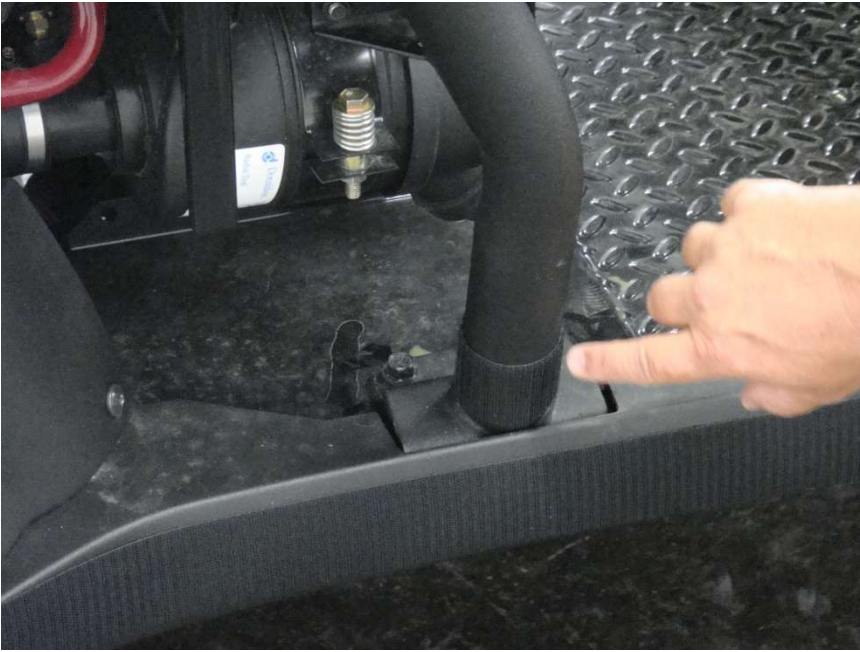
Figure 4.5 – install 6 1/2" Velcro Strip horizontally around the bottom of the Rear Roll Bar upright
