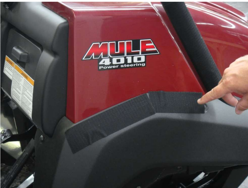
Figure 5.1 - Install the 16" Velcro Strips on the Dash Cowl / Fender Well – you will need to split the Velcro strip 10" X 6" before installing
