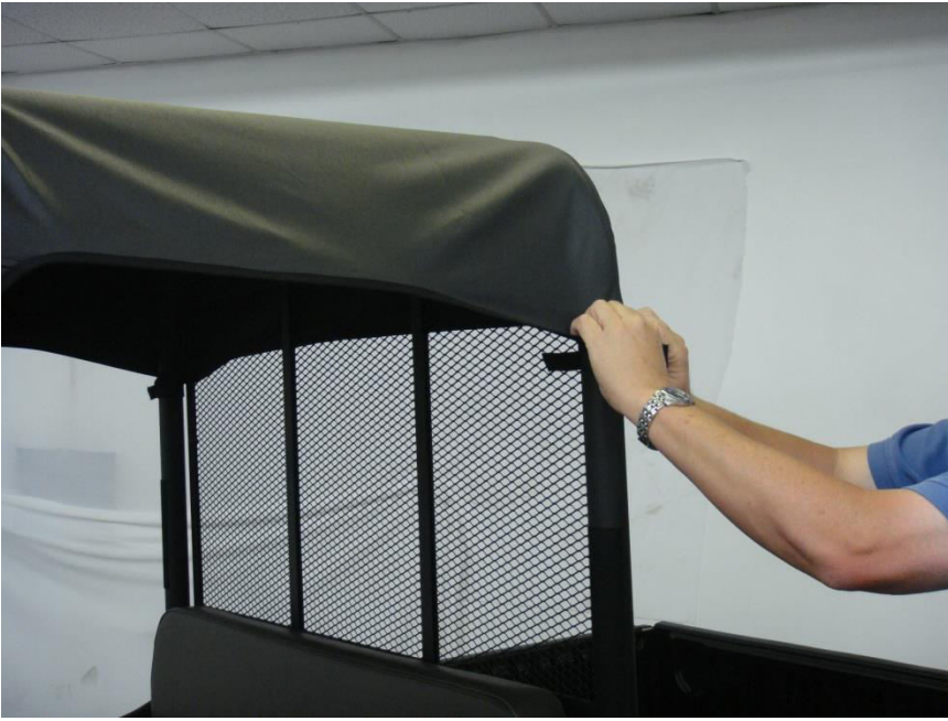
Figure 5.1 - attach Rear Roll Bar Post Velcro Tabs around installed Rear Roll Bar Velcro strips
