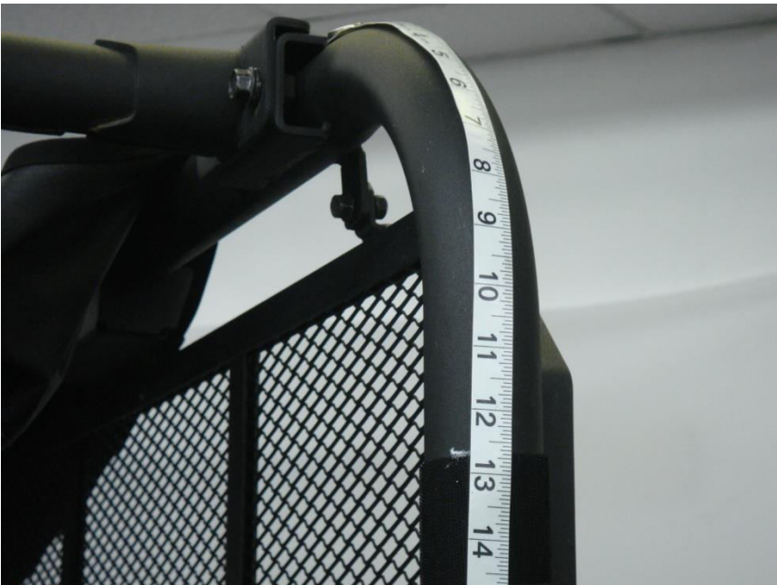
Figure 3.1 – place 6" Velcro strips horizontally around the Roll Bar Post 13" below the rear Roll Bar Cross member bolted section
