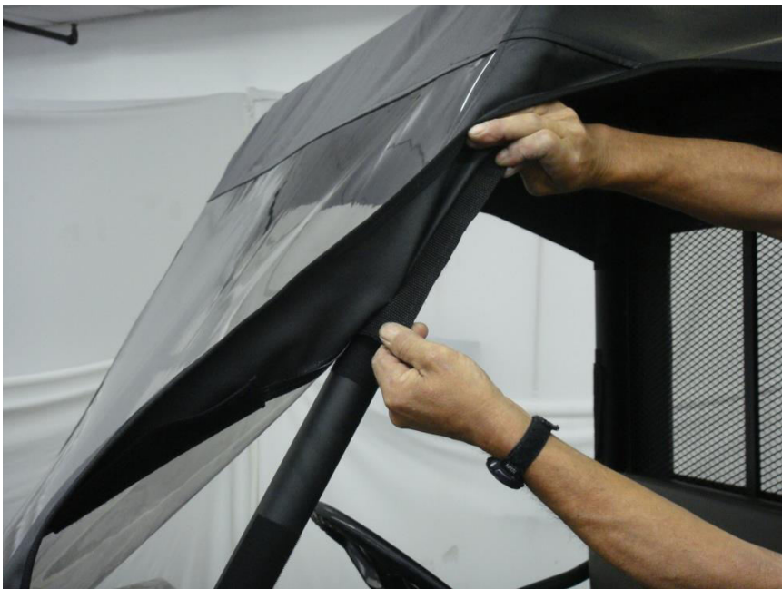
Figure 7.1 – attach top front Roll Bar Velcro Tab pulling outward and downward toward the front of the vehicle
