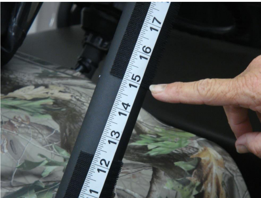
Figure 2.2 - 8" Velcro strips placed vertically 15" above the front roll bar post bolts
