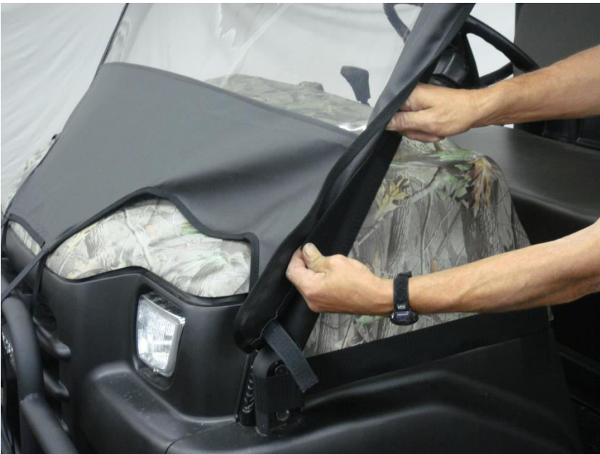
Figure 7.3 - attach lower front Roll Bar Velcro Tab pulling outward and downward toward the front of the vehicle
