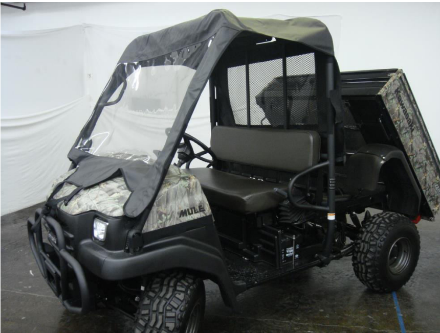
Figure 4.1 - Place enclosure loose on vehicle Cab Roll Bar Structure – Hood Straps to the front of the vehicle
