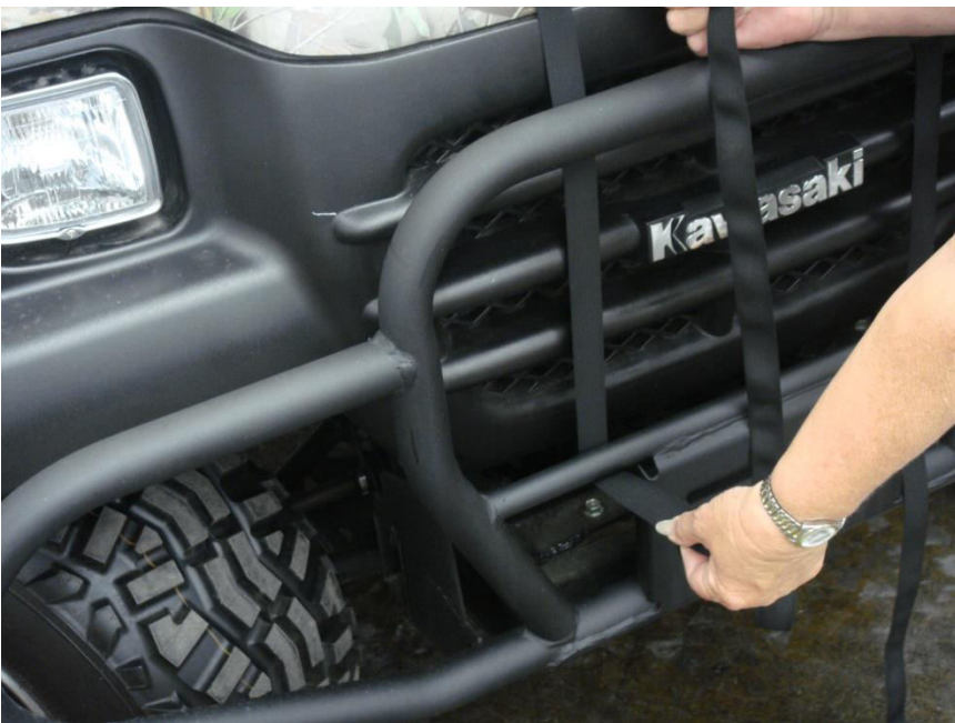
Figure 6.1 - run front hood straps through the center bar of the front bumper
