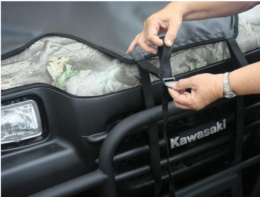
Figure 6.2 - thread front hood straps into buckles
