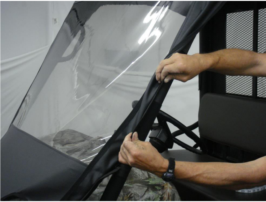
Figure 7.2 - attach middle front Roll Bar Velcro Tab pulling outward and downward toward the front of the vehicle
