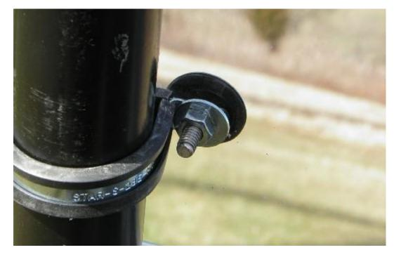
**Step 5:** To mount the upper windshield section, open 2 clamps and wrap around each of the front roll bars.
