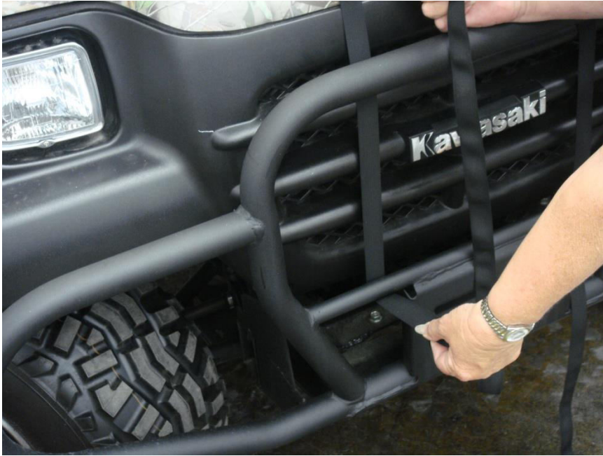
Figure 9.1 - run front hood straps through the center bar of the front bumper
