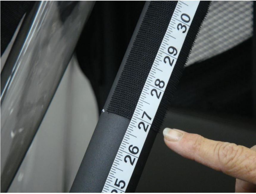
Figure 2.3 - 8" Velcro Strips placed vertically 27" above the front roll bar post bolts
