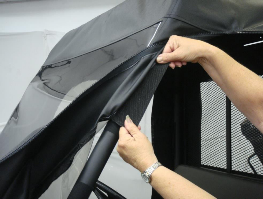
Figure 10.1 - attach top front roll bar Velcro tab
