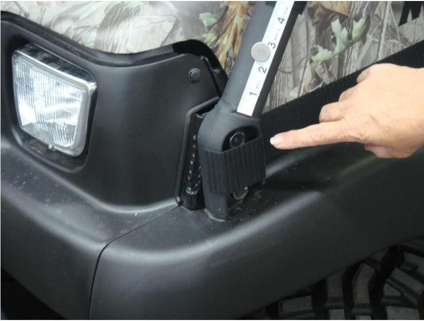
Figure 4.2 - 5" Velcro Strips placed horizontally around the front Roll Bar Bolt section
