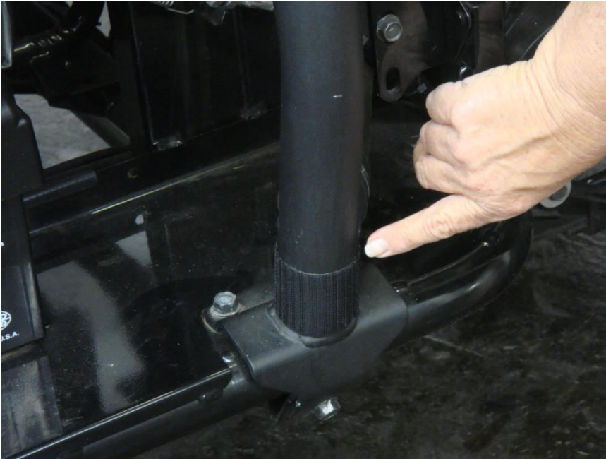
Figure 3.1 - 6" Velcro Strips placed horizontally at the base of the rear roll bar posts
