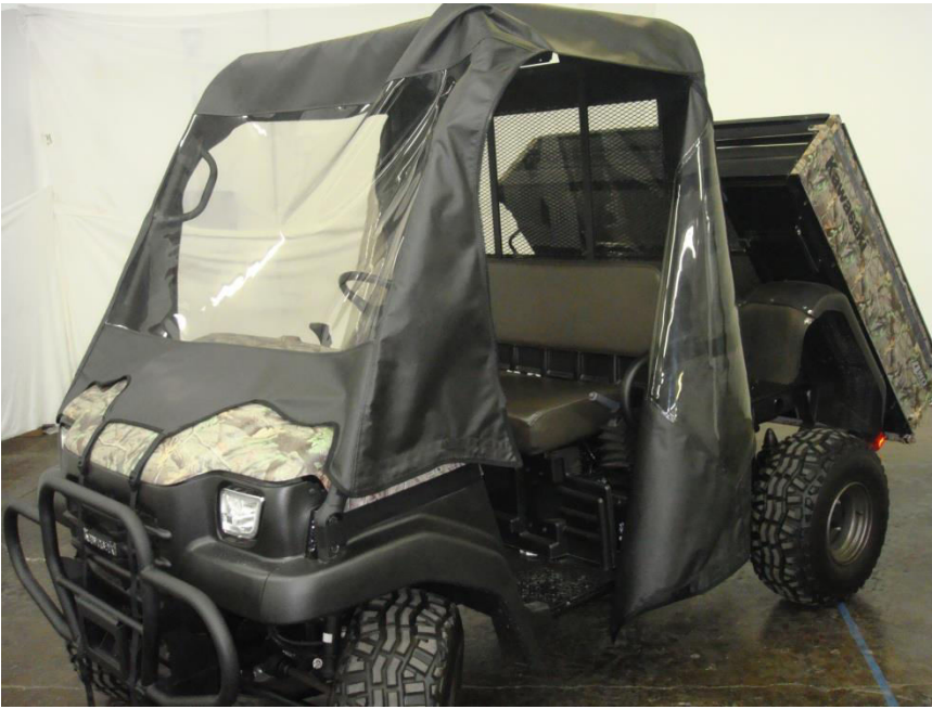
Figure 6.1 - place enclosure on vehicle cab roll bar structure
