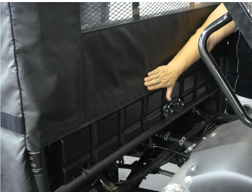
Figure 7.1 - square rear of enclosure to cab and attach rear enclosure Velcro tab to installed Velcro strip
