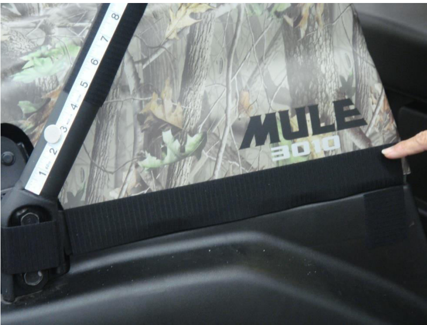
Figure 4.1 - 12" Velcro Strips placed horizontally on the side of the Dash Cowl
