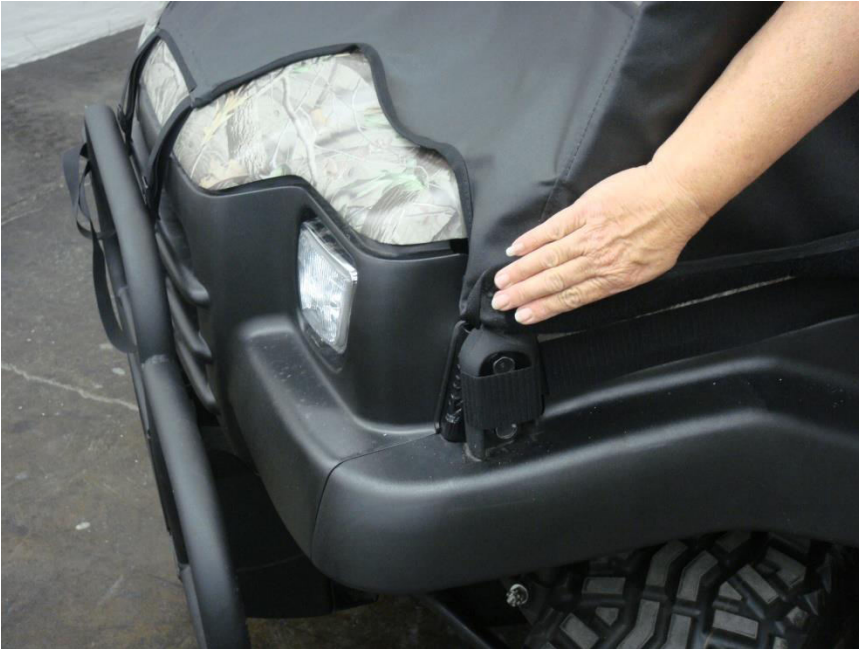
Figure 12.1 - attach Dash Cowl side Velcro Tabs
