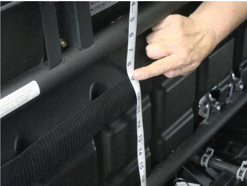
Figure 5.1 - 49" Velcro Strip Placed 9" below the top of the cab rear guard on the top raised rib
