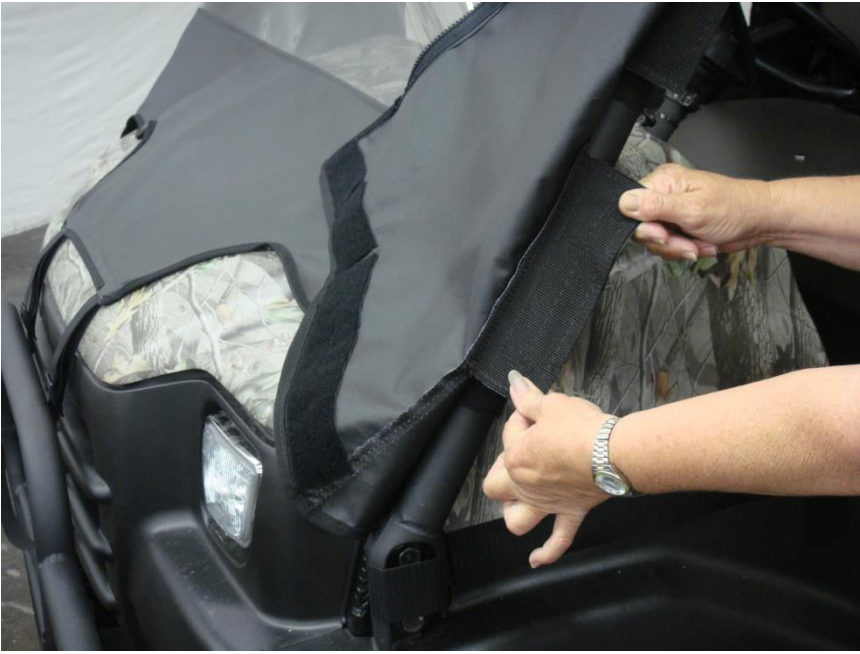
Figure 10.3 - attach bottom front roll bar Velcro tab
