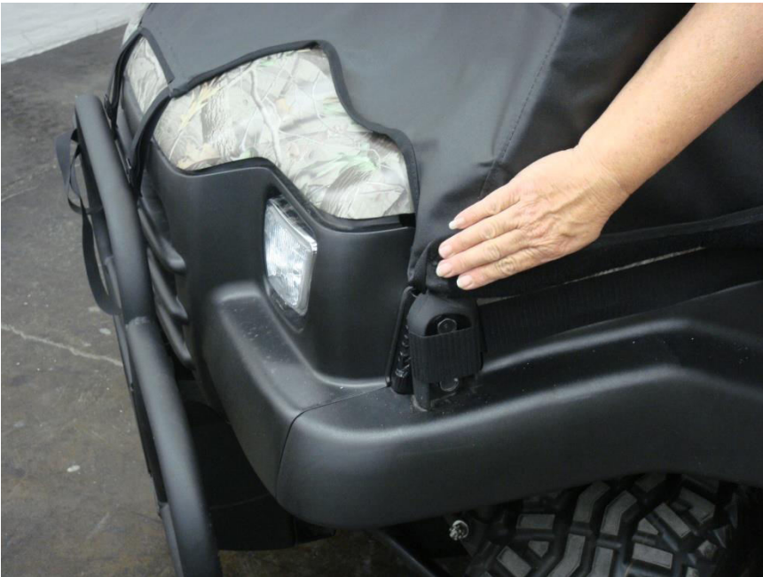
Figure 10.4 - attach front roll bar bolt section velcro
