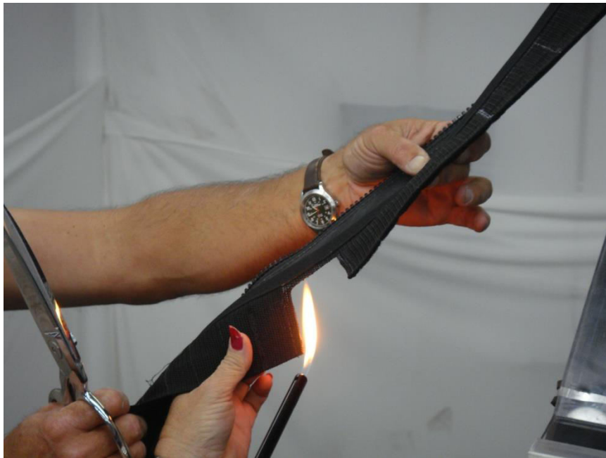
Figure 7.4 – Carefully burn the frayed thread around the cut area with a lighter.
