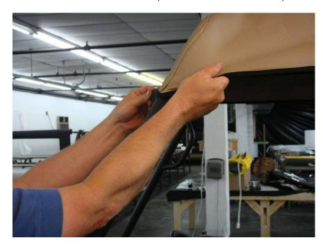
**Step 6:** Repeat all steps necessary to align and tighten the enclosure to the roll bar cage.
