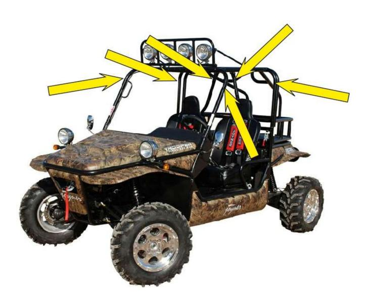
**Step 2:** Place Enclosure on top of Roll Bar Cage and align corner seams with outside center of roll bars.
