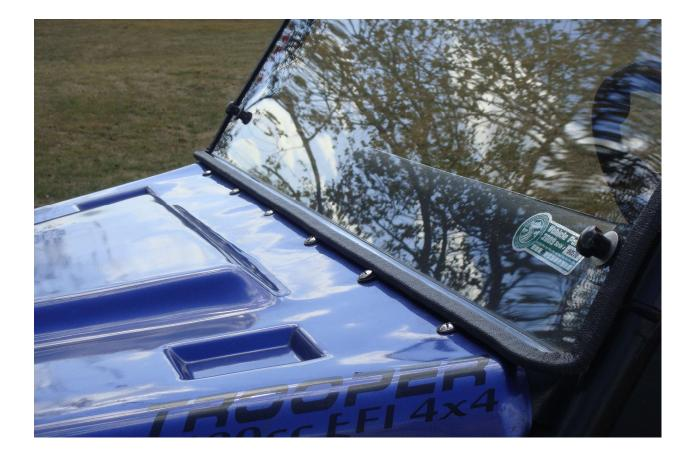
**Step 3:** Insert straps through the front of the lexan slot holes, fuzzy side facing the middle of the windshield. Wrap around the roll bar and pull back through the plastic "buckle" Pull the end of the strap tight and stick rough side to fuzzy side. Repeat for each strap.
