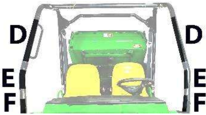
Figure 3: The tabs on the front of your doors will wrap around the front of the roll bar and attach to the Velcro strip.
