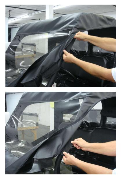
Tighten hood straps by pulling downward from the buckle on both strap ends at the same time as shown below.
