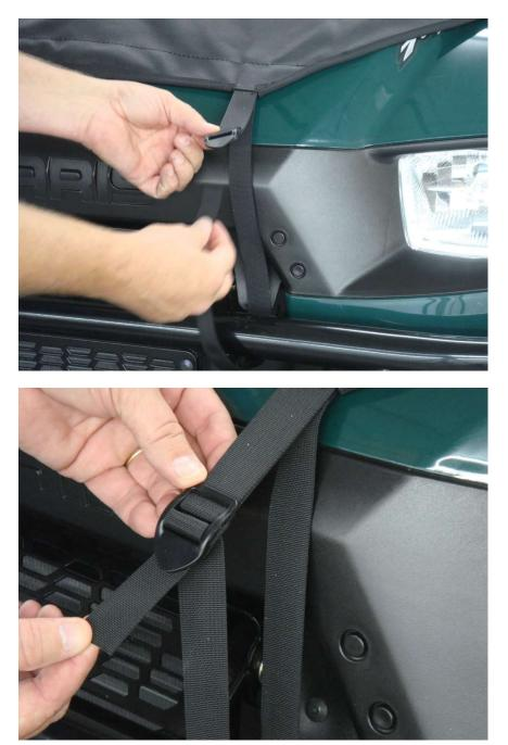
Before tightening the hood straps, make sure the windshield is square and pulled tight from side to side. Grasp the webbing/loop tabs on either side of the windshield and reposition to center and tighten the windshield as shown below.
