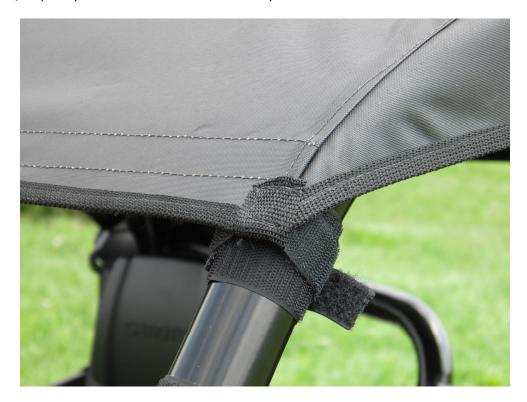
**Step 5:** Repeat any steps necessary to achieve a tight fit to the roll bar frame as shown below.
