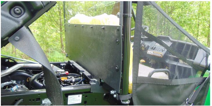
**Step 5:** Additional bolt holes have been drilled on the bottom of the lower section. The back panel should align with holes in the vehicles frame. When aligned, insert a hex head bolt with flat washer thru the bolt-hole openings in the back panel and thru the holes in the plates. Insert a nut on each bolt and tighten.
