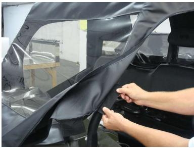
Tighten hood straps by pulling downward from the buckle on both strap ends at the same time as shown below.
