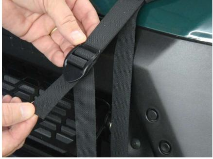
Before tightening the hood straps, make sure the windshield is square and pulled tight from side to side. Grasp the webbing/loop tabs on either side of the windshield and reposition to center and tighten the windshield as shown below.
