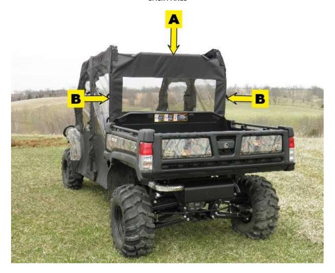
**Step 4:** After all adhesive hook strips are attached, begin attaching the enclosure to the cab frame. As you attach the hook and loop, square each panel to the frame. **PLEASE NOTE, FOR MAXIMUM ADHESION, ALLOW THE ADHESIVE HOOK TO ADHERE TO THE FRAME FOR 24 HOURS BEFORE PULLING AGAINST THE HOOK WITH THE LOOP STRIPS.**
