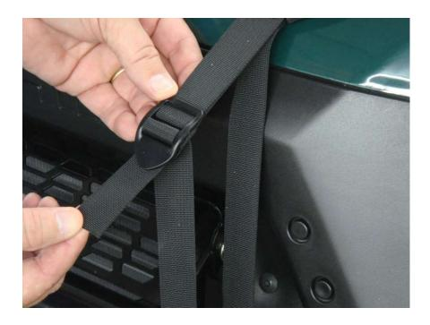
Tighten front hood straps by pulling downward from the buckle on both strap ends at the same time as shown below. DO NOT FULLY TIGHTEN UNTIL THE TENSION STRAP ON THE BACK OF THE WINDSHIELD/TOP IS IN PLACE.
