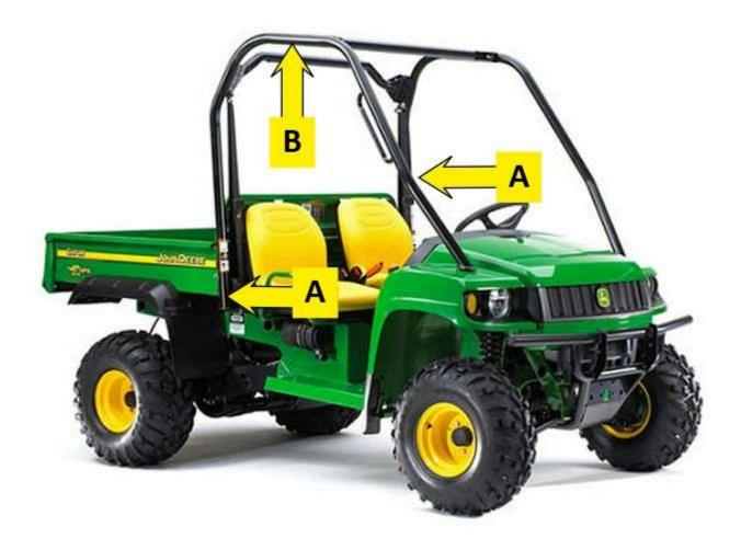
**Step 3:** With the adhesive hook strips in place, place the top loosely on top of the vehicle roll cage making sure the enclosure front visor is facing toward the front of the vehicle. Align the side seams with the outside edge of the roll bars.
