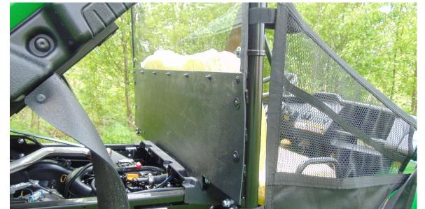
**Step 3:** One at a time, open a clamp and wrap around the rear roll bars. The flat side of the loop clamps should face to the rear with the bolt hole openings on the inside of the roll bars. The clamps will not stay in place until bolted to the pack panels. However, the final location of the clamps are shown in the following picture.
