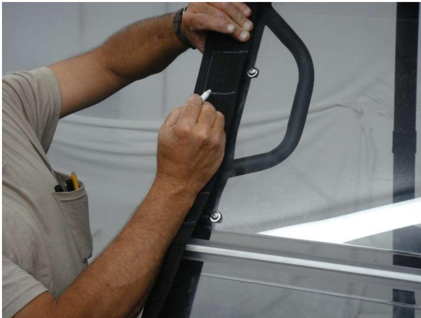
**Step 3: Cut a section out around where your clamps will be positioned on the Velcro tab as shown. Be careful not to cut the binding.**
