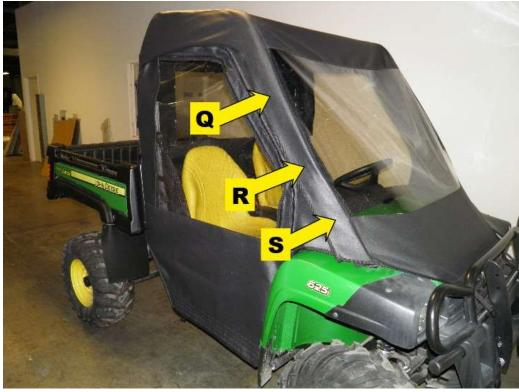
**Step 3:** After all adhesive hook strips are attached, begin attaching the enclosure to the cab frame. As you attach the hook and loop, square each panel to the frame. **PLEASE NOTE, FOR MAXIMUM ADHESION, ALLOW THE ADHESIVE HOOK TO ADHERE TO THE FRAME FOR 24 HOURS BEFORE PULLING AGAINST THE HOOK WITH THE LOOP STRIPS.**
