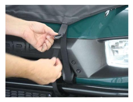
Bringing the end of the straps up to the latch buckle, run the end through the back of the top buckle opening first and then through the front of the lower buckle opening as shown.
