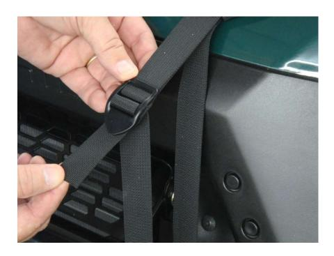
Tighten front hood straps by pulling downward from the buckle on both strap ends at the same time as shown below. **DO NOT FULLY TIGHTEN UNTIL THE TENSION STRAP ON THE BACK OF THE WINDSHIELD/TOP IS IN PLACE.**
