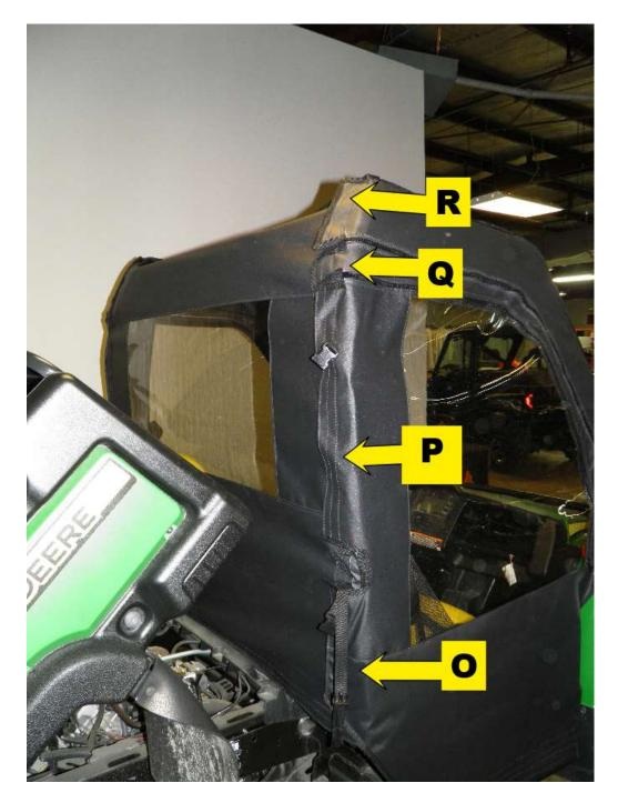
**Step 3:** After all adhesive hook strips are attached, begin attaching the enclosure to the cab frame. As you attach the hook and loop, square each panel to the frame. **PLEASE NOTE, FOR MAXIMUM ADHESION, ALLOW THE ADHESIVE HOOK TO ADHERE TO THE FRAME FOR 24 HOURS BEFORE PULLING AGAINST THE HOOK WITH THE LOOP STRIPS.**
