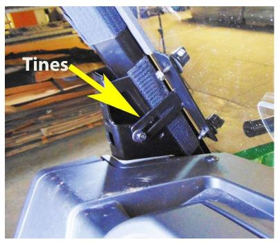
**Step 3:** Place lower windshield on UTV. Line up the slots in the lexan with the slots in the metal bracket. You will notice that the lexan is flat and the UTV is slightly curved, that is ok you will push the windshield down into place and insert a bolt, wingnut, and neoprene washer (pictured below) into the front of the lexan and through the slot in the metal bracket. Secure with small washer and nut. DO NOT TIGHTEN ALL THE WAY. Install all bolt, wingnut, and neoprene combinations first.
