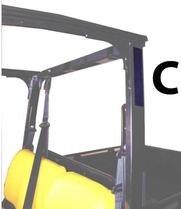
Figure 3: Shows placement of 10" Velcro strip C.
