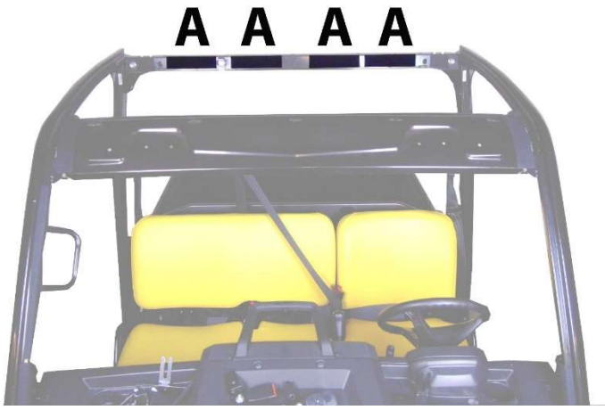
Figure 2: Shows placement of 8" Velcro strips A.
