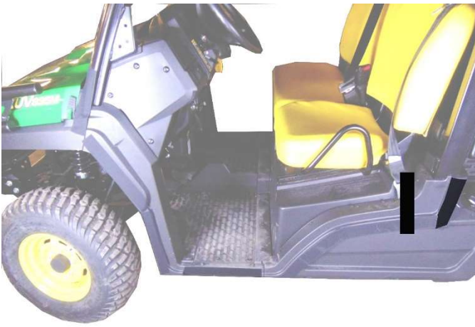
Figure 7: Shows placement of 9" Velcro strip I.
