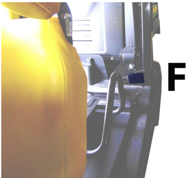
Figure 5: Shows placement of 3" Velcro strip F. Raise seat all the way up and place strip under the seat belt roll.
