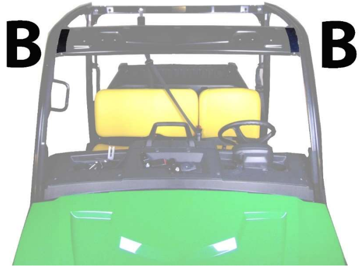
Figure 2: Shows placement for 8" Velcro strip B.
