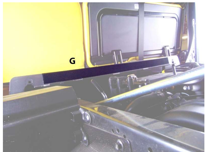
Figure 6: Shows placement of 34" Velcro strip G. Raise bed, attach to the flat bracket behind the seat.
