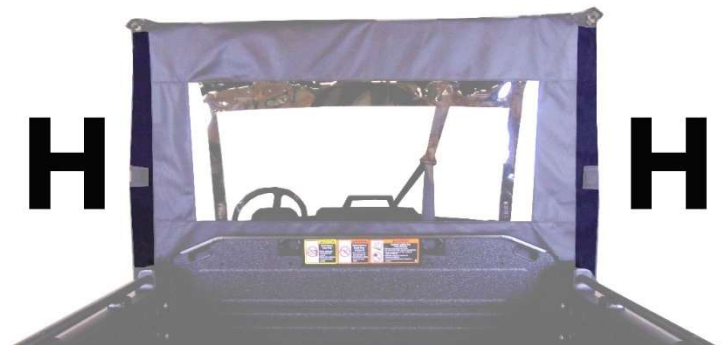
Figure 6: Shows placement of Velcro on the back panel, if you only purchased a door kit then you will place this strip on the roll bars from the top all the way down the back of the roll bars. If you have a back panel you will not need this Velcro. If you have a lexan back panel, the adhesive Velcro is optional, the lexan back panel will go over the door panels Velcro tabs, tightening the Lexan back panel into place will hold your doors to the UTV frame.
