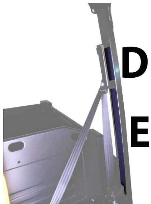
Figure 4: Shows placement of 7" Velcro strip D and 22" Velcro strip E.
