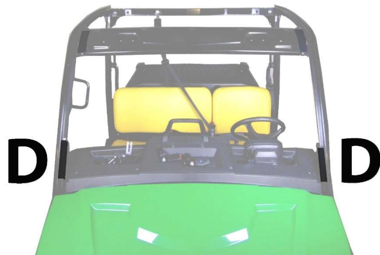
Figure 4: Shows placement of 7" Velcro strip D. This strip should rest in a similar position to strips in Figure 3. If you have a windshield the strip will set underneath the clamps.
