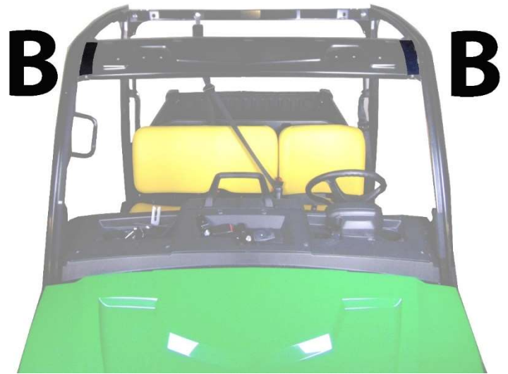
Figure 2: Shows placement for 8" Velcro strip B.
