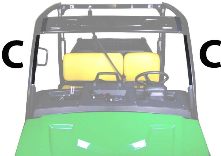
Figure 3: Shows placement for 18" Velcro strip C. Strips should rest on inset roll bar fold down on to interior edge.
