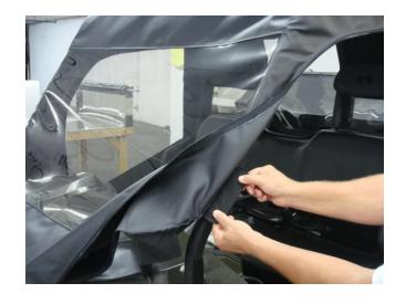
**Step 6:** Tighten hood straps by pulling downward from the buckle on both strap ends at the same time as shown below.
