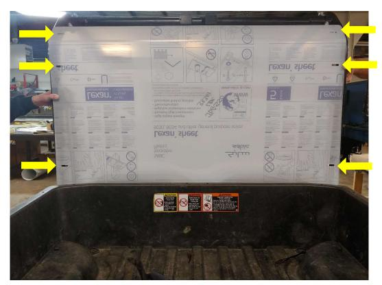
**Step 3:** With the included hardware fasten the back panel to the roll bars with the loop clamps as shown below.
