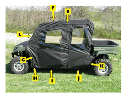
**Step 4:** After all adhesive hook strips are attached, begin attaching the enclosure to the cab frame. As you attach the hook and loop, square the enclosure to the frame. The adhesive strips that run the length of the front roll bars must be cut to accommodate the windshield clamps. Follow the instructions accordingly.
