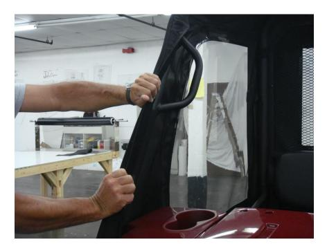
**Step 7:** The webbing/Velcro strip that runs the length of the front roll bars will need to be cut to accommodate the windshield clamps and the grab handle. With chalk, mark the webbing strip where cuts will be made. **DO NOT CUT INTO THE BINDING.**
