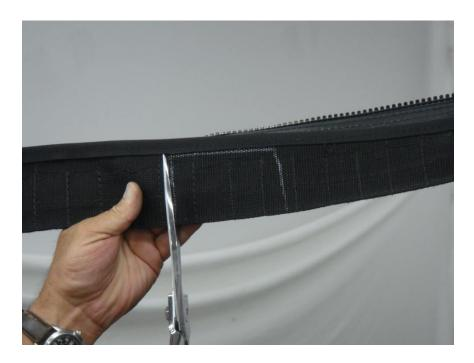
Cut the Tab being very careful not to cut the binding at the edge.
