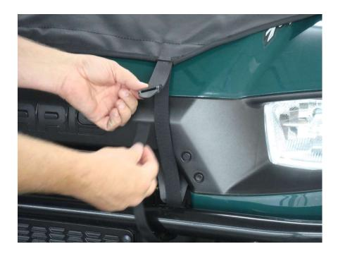
**Step 5:** Before tightening the hood straps, make sure the windshield is square and pulled tight from side to side. Grasp the 8" webbing/loop tabs on either side of the windshield and reposition to center and tighten the windshield as shown below.
