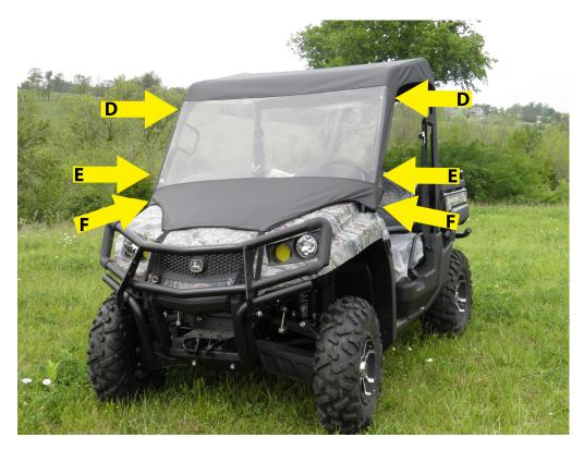
**Step 3:** After all adhesive hook strips are attached, begin attaching the enclosure to the cab frame. As you attach the hook and loop, square the enclosure to the frame. **PLEASE NOTE, FOR MAXIMUM ADHESION, ALLOW THE ADHESIVE HOOK TO ADHERE TO THE FRAME FOR 24 HOURS BEFORE PULLING AGAINST THE HOOK WITH THE LOOP STRIPS.**
