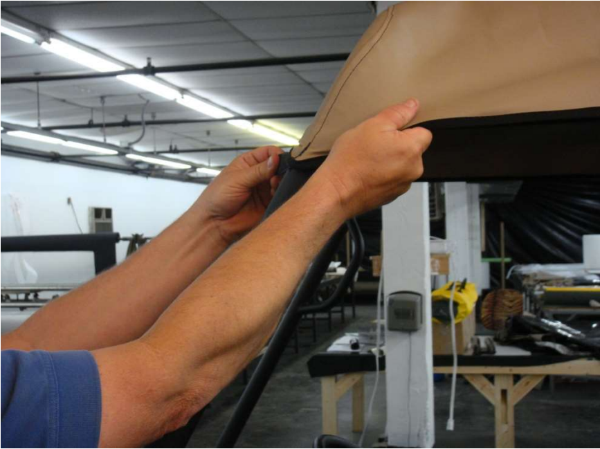
Figure 5.1 - Attach front and rear Enclosure Velcro tabs to installed Velcro strips
