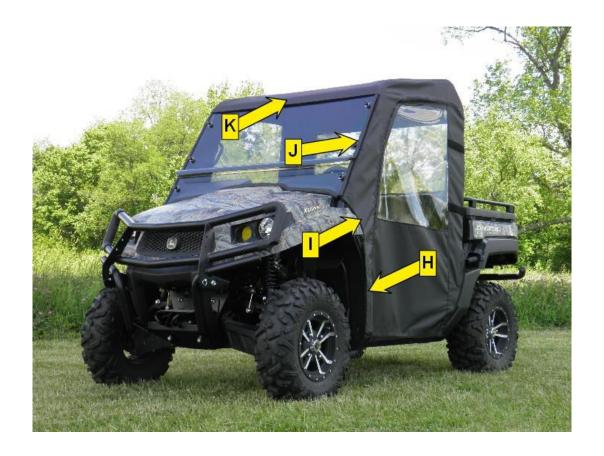
**Step 4:** After all adhesive hook strips are attached, begin attaching the enclosure to the cab frame. As you attach the hook and loop, square the enclosure to the frame. **PLEASE NOTE, FOR MAXIMUM ADHESION, ALLOW THE ADHESIVE HOOK TO ADHERE TO THE FRAME FOR 24 HOURS BEFORE PULLING AGAINST THE HOOK WITH THE LOOP STRIPS.**
