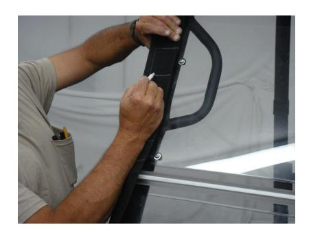
**Step 6:** Cut the webbing strip with household scissors. **AGAIN, DO NOT CUT INTO THE BINDING.** Seal the frayed edges with a lighter. Have a wet cloth handy to dab the edges if needed.
